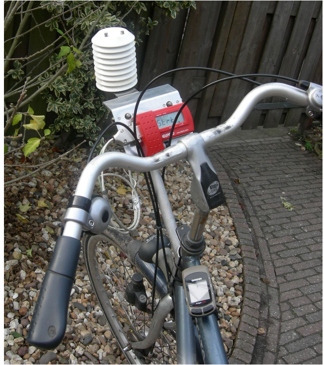
Figure 2: Mounting of the instruments in front of the bike. The orange part is the datalogger with a display, the temperature and humidity sensors are in the multi-plated screen. The GPS is visible on the horizontal bar of the bike.
