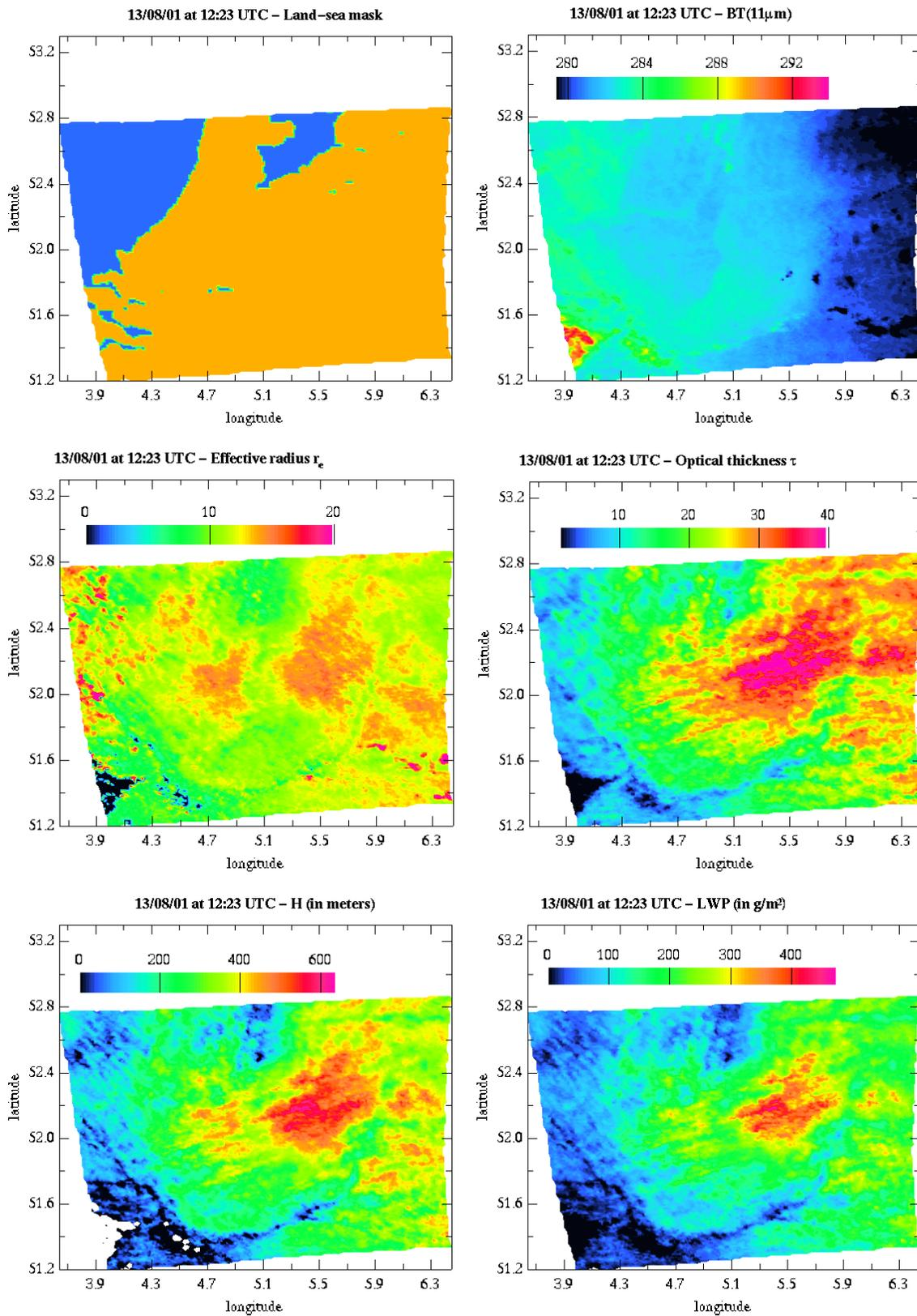
Figure 6.1 Analysis of ATSR measurements from the ERS platform on 14 August 2001 at 12:23 UTC.
