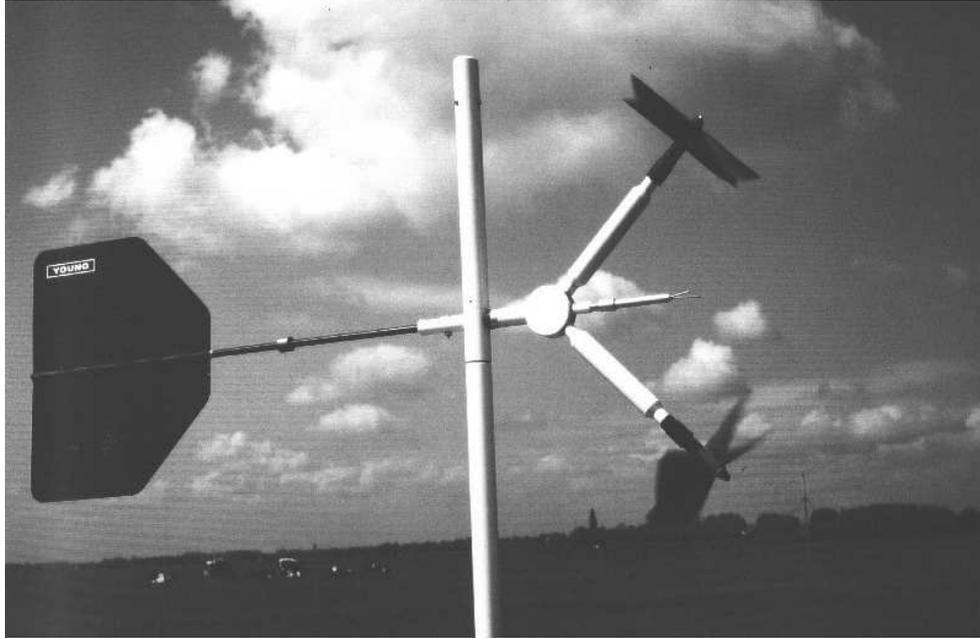
Figure 2.1: Picture of the K-Gill Propeller Vane.
