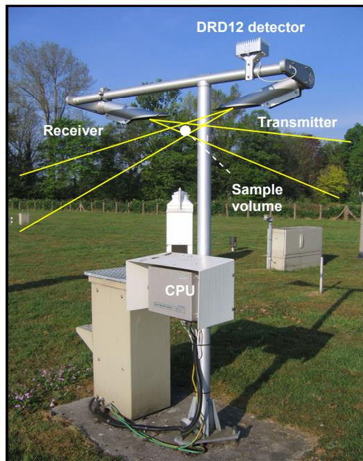
Figure 1.1. The Vaisala FD12P weather sensor in De Bilt (station 260).
