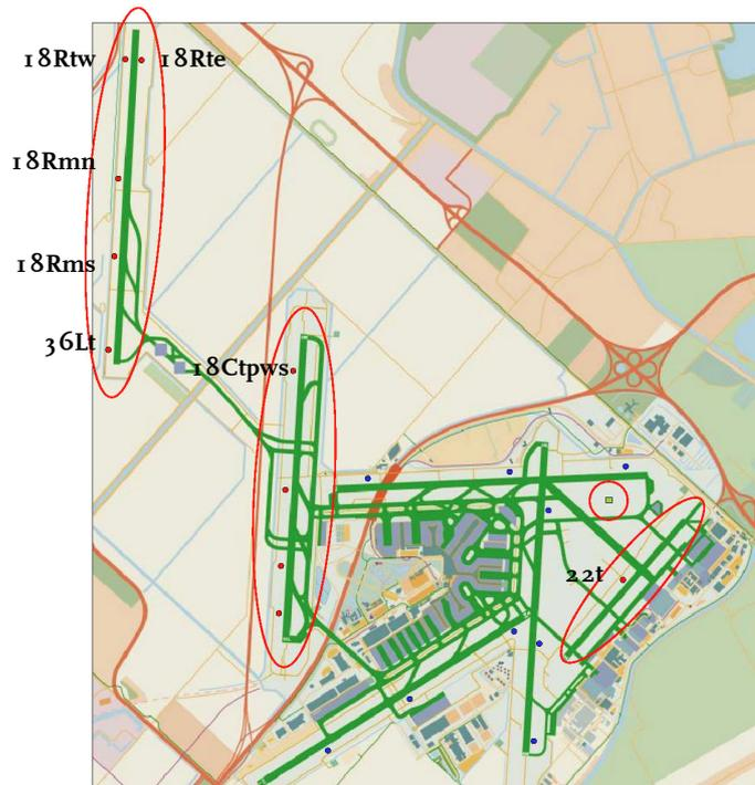
Figure 5.1. Overview of locations of sensors at Schiphol airport. The green square indicates the observation field and a red or blue dot represents a FD<sub>12P</sub> sensor or transmissometer, respectively.
