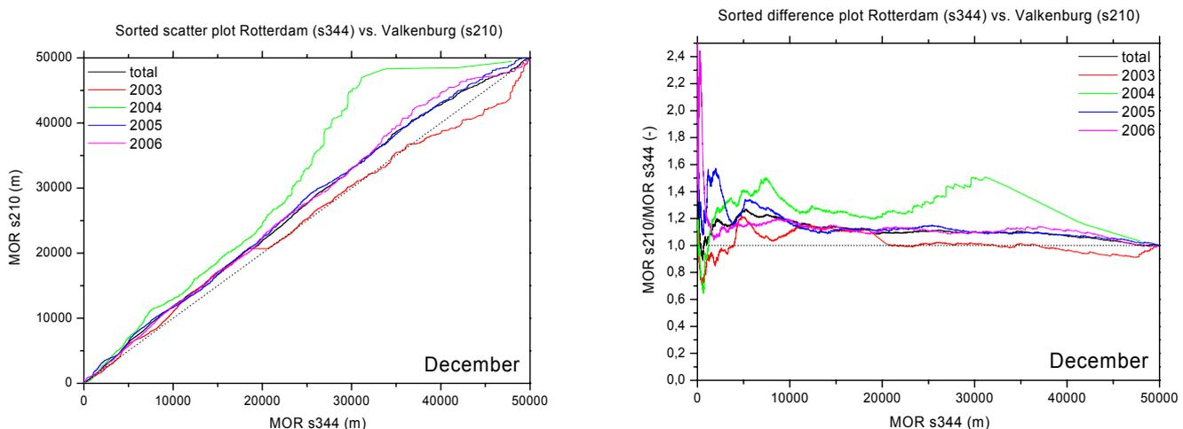
Figure 4.10. Sorted scatter plots of the 10-minute automated MOR observations in Rotterdam (344) versus Valkenburg (210), December 2003-2006. The ratio of the MOR values in the sorted plot is presented in the right panel.
