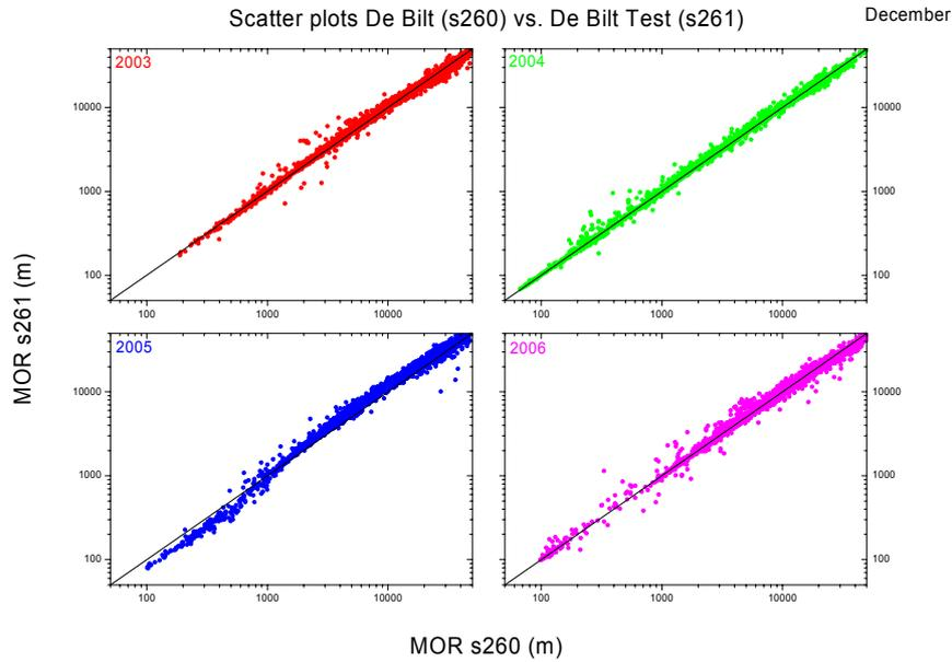
Figure 4.7. Scatter plot of the 10-minute automated MOR observations for the FD 12Ps at De Bilt 260 versus 261, December 2003-2006.
