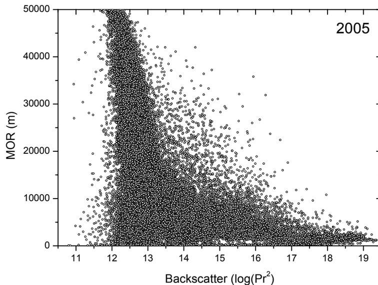
Figure 4.11. Ceilometer backscatter at the lowest available gate versus MOR at station 261 for the year 2005. Both parameters are presented on a 10-minute basis.
