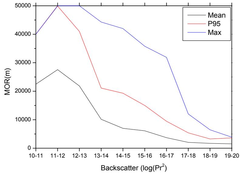
Figure 4.12. Mean, 95% and maximum MOR values for 10 ranges of LD-40 backscatter at station 261 for the year 2005.
