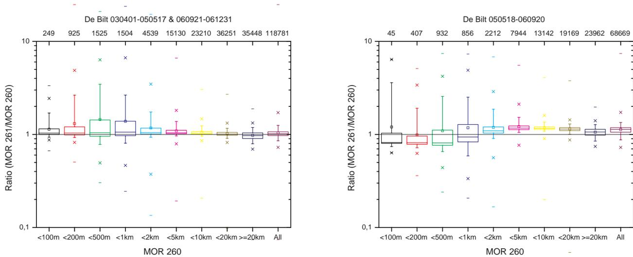
Figure 4.9. Box plots of the ratio of 10-minute MOR measurements for the FD12Ps at De Bilt 260 and 261. The sensors have the same software version in the left panel, in the right panel the sensor at 261 has an updated calibration curve. Legend: ‘-’ = min/max, ‘x’ = 1/99%, ‘□’ = mean, the box indicates the 25/75% boundaries, the whiskers extended from the box indicate 5/95% and the line in the box represents the median.
