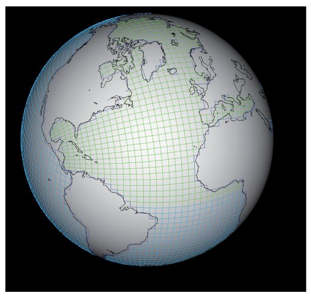
Fig. 4. The horizontal grid of the model at a resolution of 3° by 3°. The view is centred on the Atlantic. The two spherical subgrids in two different colors are connected in the Atlantic at the "geographical equator".
