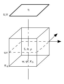
Fig.3. Location of the various variables on the grid of CLIO. U,V are the two components of the barotropic velocity,  $\eta$  the surface elevation, u, v, w, the three components of the velocity, S the salinity,  $\theta$  the potential temperature,  $q^2$  (two times) the turbulent kinetic energy,  $K_s$  and  $K_u$  the vertical diffusion and vertical viscosity.
