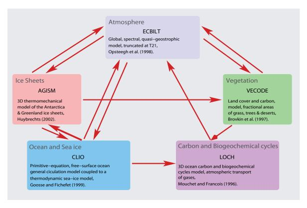
Fig. 1. Sketch of the LOVECLIM model showing the interactions between the five components.
