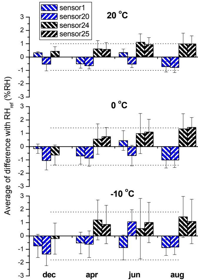
Figure 6. On the y-axes: average deviation of the difference between the sensor and the reference (in %RH) of the sensors indicated (blue: HMT 337, black: EE 33) for the different temperatures (20, 0 and -10 °C) and series (dec, apr, jun and aug). The standard deviation for each series is indicated by the error bar, the dashed line the uncertainty of the measurement for the temperature in question.
