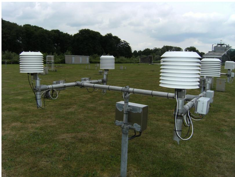
Figure 4. The field test in De Bilt. Shown are the radiation screens containing the humidity sensors.
