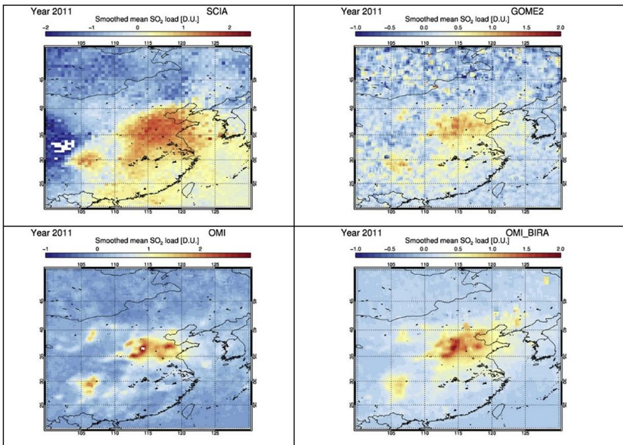
Fig. 2. Yearly smoothed  $\text{SO}_2$  load [D.U.] over Eastern China in 2011. **Upper left:** SCIAMACHY/Envisat; **upper right:** GOME2/MetopA; **lower left:** OMI\_NASA/Aura and **lower right:** OMI\_BIRA/Aura. Not the slightly altered colour scale to accommodate the different  $\text{SO}_2$  load ranges. (For interpretation of the references to colour in this figure legend, the reader is referred to the web version of this article.)
