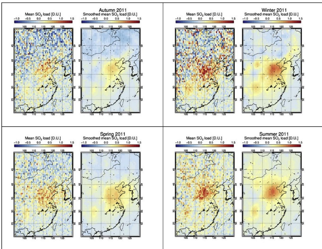
Fig. 1. Seasonal mean SO<sub>2</sub> loads [left panels] and smoothed mean SO<sub>2</sub> loads [right panels] for the GOME2/MetopA product in autumn [top left], winter [top right], spring [bottom left] and summer [bottom right] are shown.
