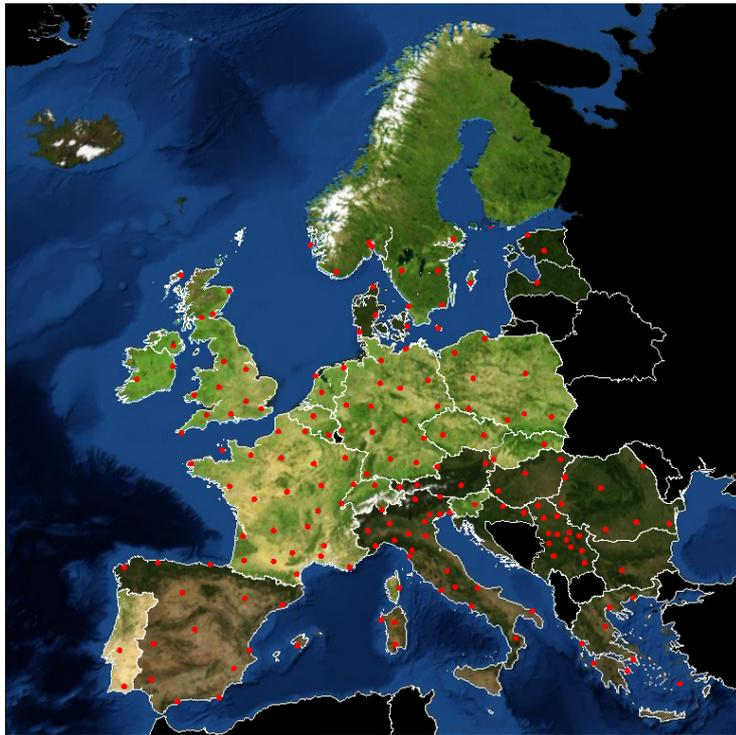
Figure 2.1. Radars (red dots) available within the OPERA network (green colored countries). The bright countries delivered data for the FlySafe2 project described in this report.
