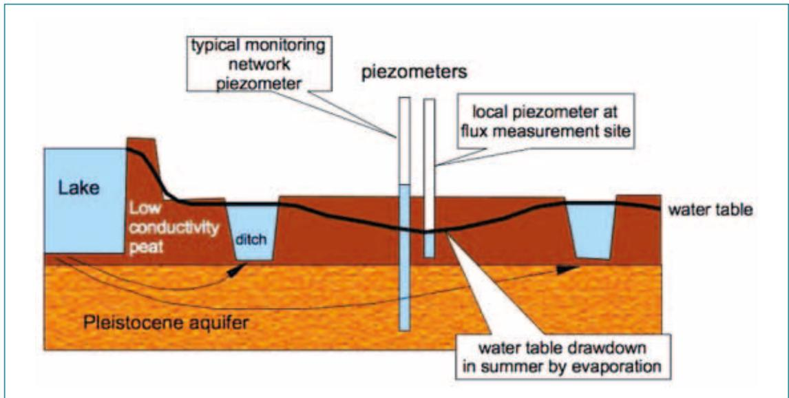
Figure 11. Small-scale spatial variation in groundwater table which is not recorded by groundwater models.
