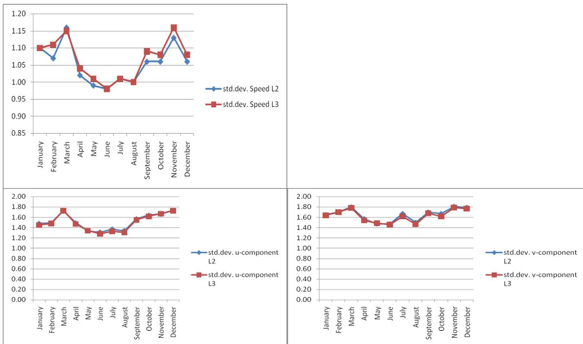
Figure 6 Buoy collocation results for L2 and L3 ASCAT 25km windproduct over 2009: average standard deviation of speed (top) and u and v-component (bottom).
