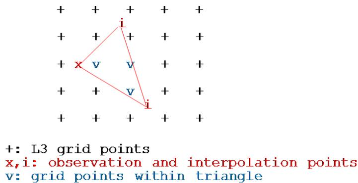
Figure 2 Illustration of gridpoints that are filled with bilinear interpolated values of  $u$  and  $v$  in the triangle spanned up by an observation point (WVC) and two interpolated observation points.
