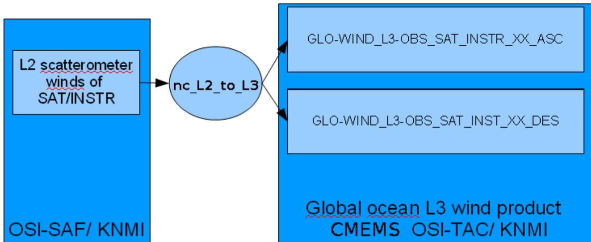
Figure 1 Schematic view of the L3 processing procedure for scatterometer "INST" on satellite "SAT".
