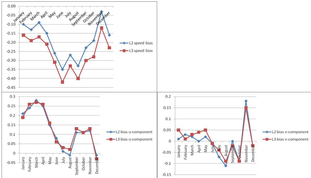
Figure 5 Buoy collocation results for L2 and L3 ASCAT 25km windproduct over 2009: average bias of speed (top) and u and v-component (bottom).
