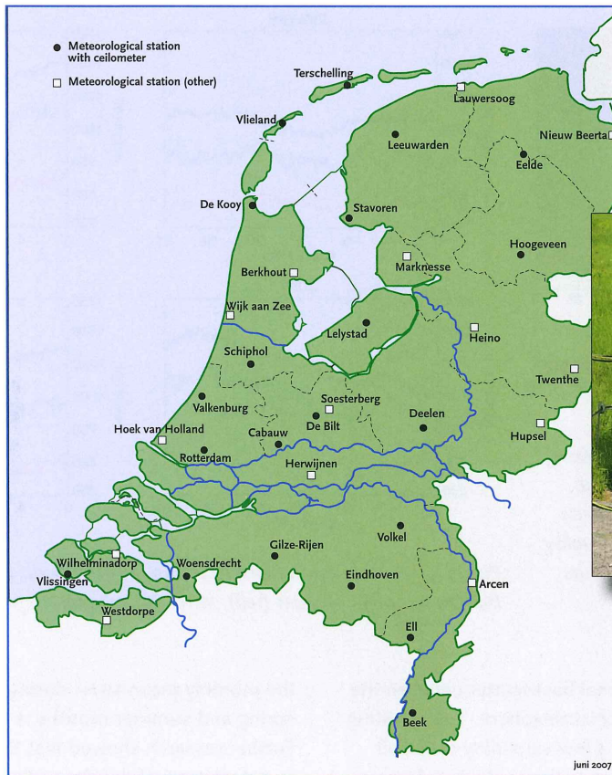
Figure 1. Map of the KNMI meteorological observation network in The Netherlands. The locations with a LD-40 ceilometer (inset photograph) are represented by black dots.
