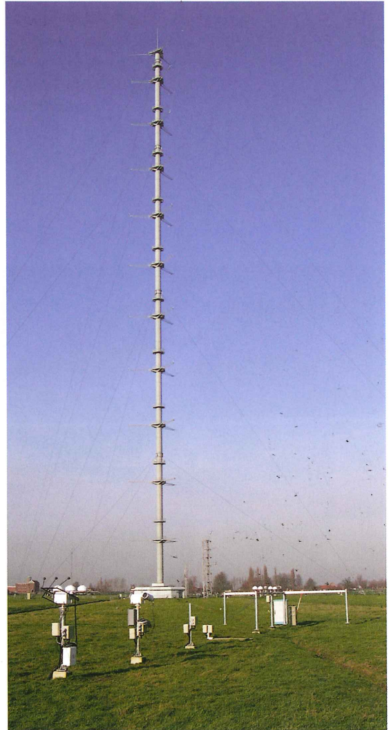
Figure 2. Photographs showing the BSRN station and the 200 m tower in Cabauw. The basic radiation measurements consist of global, direct, diffuse and downward longwave radiation. In addition, various spectral solar radiation measurements are made. Images of the sky are made using a Total Sky Imager. Photographs taken by W.H. Knap, January 2005.
