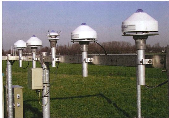
Figure 2. Photographs showing the BSRN station and the 200 m tower in Cabauw. The basic radiation measurements consist of global, direct, diffuse and downward longwave radiation. In addition, various spectral solar radiation measurements are made. Images of the sky are made using a Total Sky Imager. Photographs taken by W.H. Knap, January 2005.
