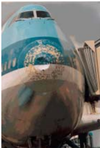
Figure 1. KLM airplane at Amsterdam Airport Schiphol damaged by large hail.
