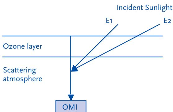
Figure 3. Principle of zenith sky measurements. At two solar elevations, E1 and E2, the path through the absorbing ozone layer differs and the ratio of these spectra will correspond to the absorption spectrum of ozone.
