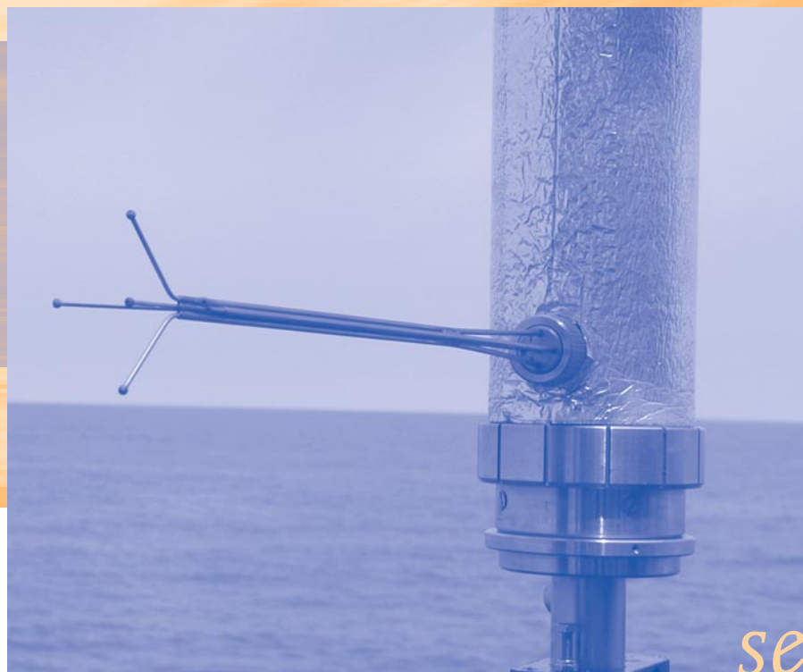
Figure 4. Photograph showing a pressure anemometer (PA). The version of the PA shown here was constructed especially for use on the wave follower. The flow outlet tubes can clearly be seen.
