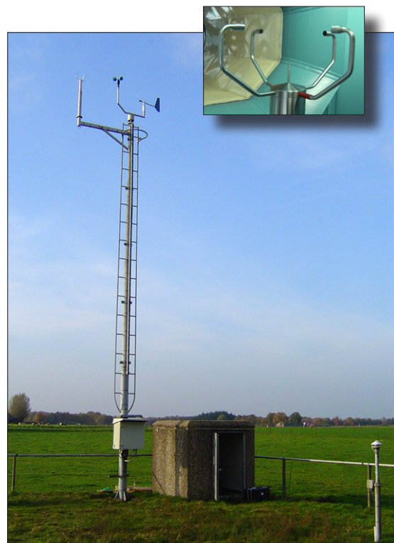
Figure 1. The wind mast at Hupsel equipped with a sonic wind sensor and the operational KNMI cup anemometer and wind vane. The inset shows the Thies 2D sonic.
