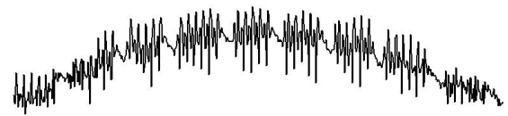
Figure 4. Wingbeat pattern of a small songbird with regular phases of wingbeats (frequency around 15 Hz) and pauses as recorded by the Superfledermaus bird radar. The single wingbeats are clearly visible. The envelope of increasing and decreasing amplitude (vertical axis) of the signal along the time axis (horizontal axis) reflects the bird's flight entering the radar beam at one edge, flying through the centre and leaving at the other edge.
