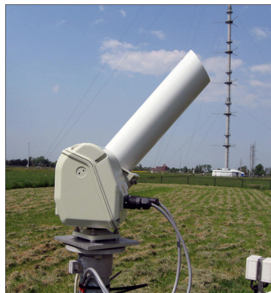
Figure 6. The NubiScope at the Baseline Surface Radiation Network (BSRN) site of Cabauw.
