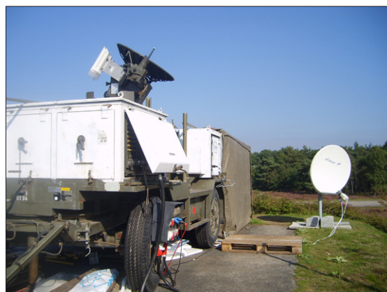
Figure 3. The bird radar Superfledermaus equipped with a camera mounted parallel to the radar antenna.
