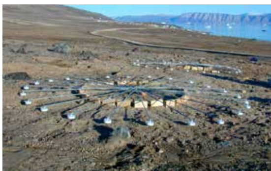
◀ Measuring instrument IS18 is the infrasound array in Greenland. Source: CTBTO Public Information
