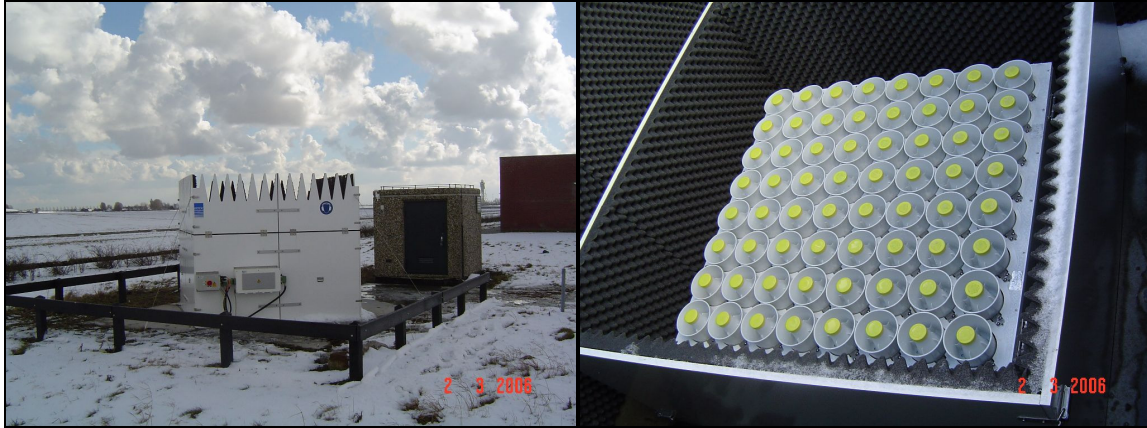
Figure 1. The METEK SODAR at Schiphol Airport. The SODAR PC is installed in the small building next to the instrument. In the right-hand panel a close-up of the array with 64 loudspeakers is shown.
