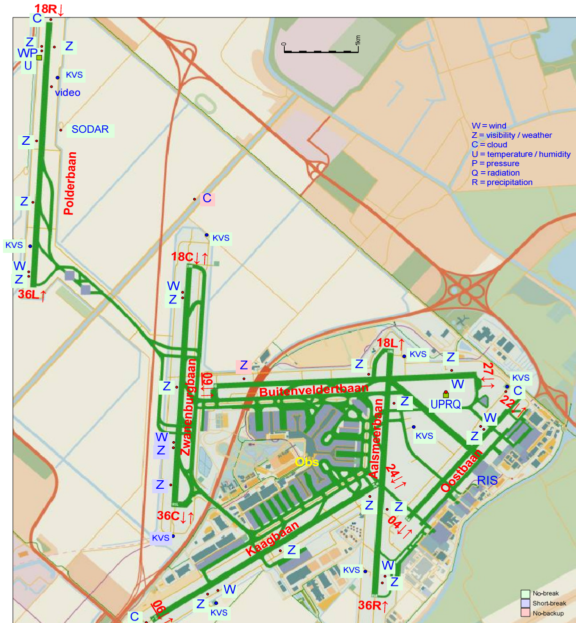
Figure A.1. Overview of meteorological sensor locations at Schiphol Airport (courtesy: W. Wauben). The legend in the upper right corner describes the parameter abbreviations. Note that the SODAR is located about halfway and 200 m east of the Polderbaan (18R-36L). Ceilometers (indicated by "C") are situated close to the touchdown zones of runways 18R, 18C, 06 and 27.
