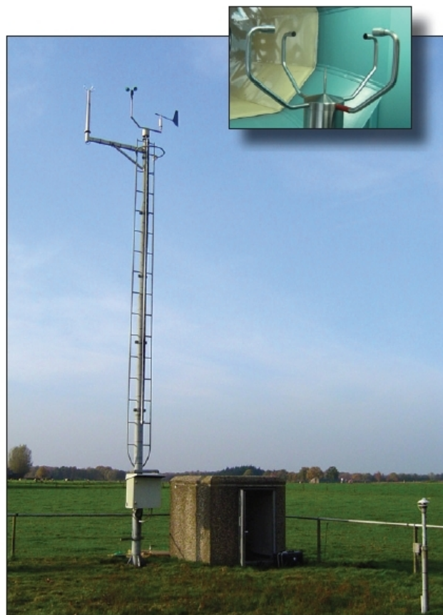
Figure 1. The wind mast at Hupsel equipped with a sonic wind sensor and the operational KNMI cup anemometer and wind vane. The inset shows the Thies 2D sonic.
