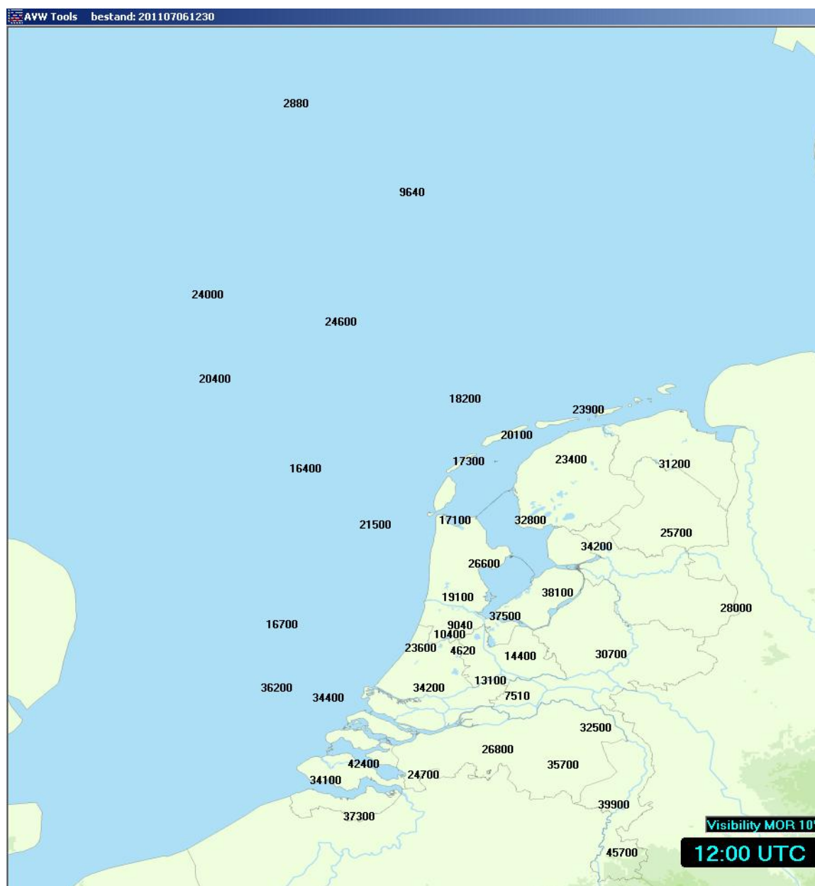
Figure 15: Illustration of the MetNet visibility information in The Netherlands that is centrally available and can be visualized geographically with an update every 10 minutes.
