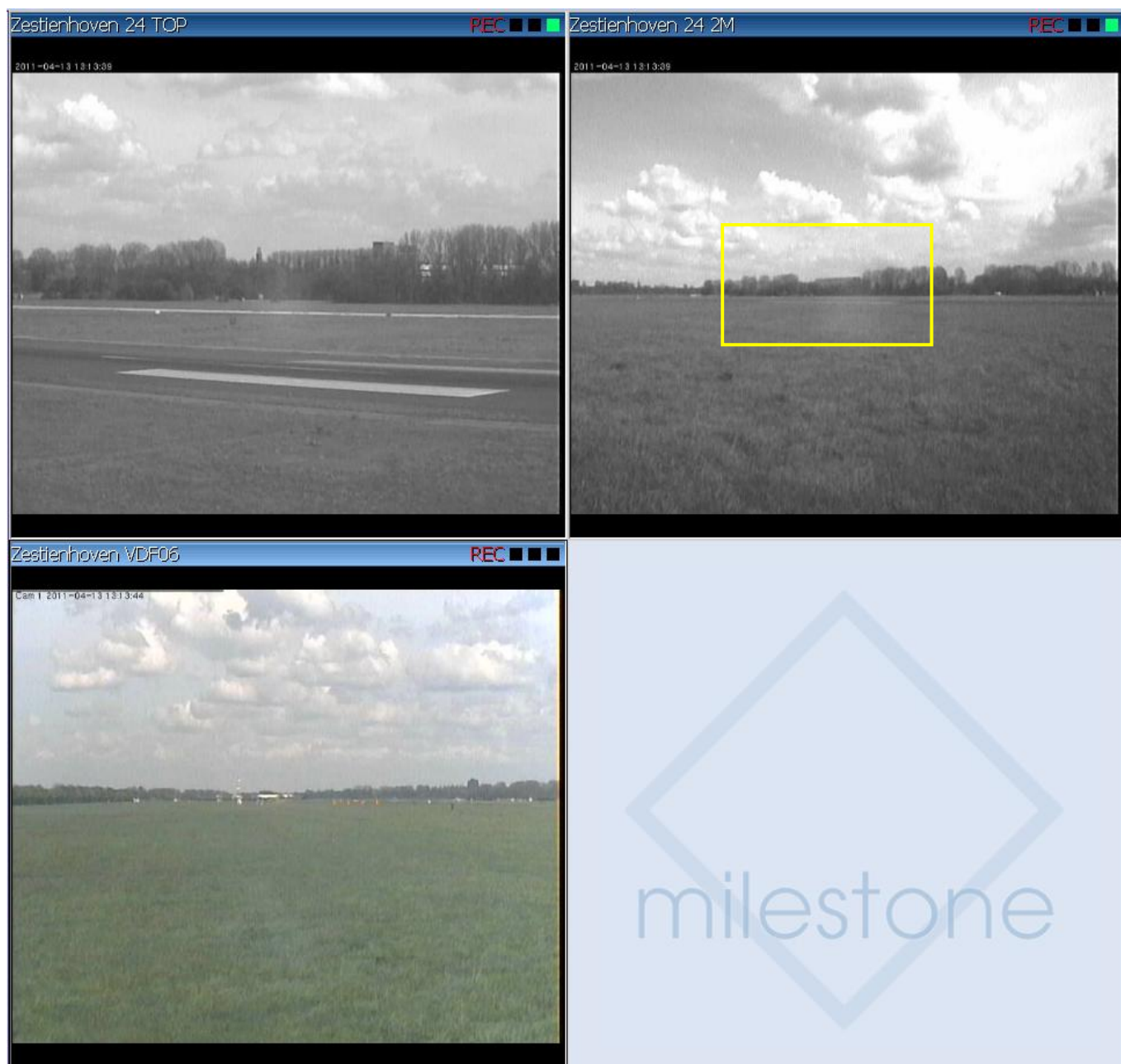
Figure 13: Illustration of the images obtained with the video cameras at 24 touchdown at Rotterdam The Hague Airport (top panels) and the camera before the threshold of runway 06. The yellow rectangle indicates the field of view of the video camera at 9 m equipped with a tele lens in the image obtained with the video camera at 2 m equipped with a wide-angle lens.
