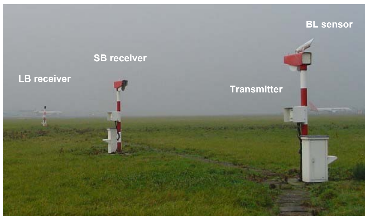
Figure 1: The Vaisala MITRAS transmissometer with the transmitter equipped with background luminance sensor in the foreground (right), the short baseline receiver (middle), and the long baseline receiver in the background (left).
