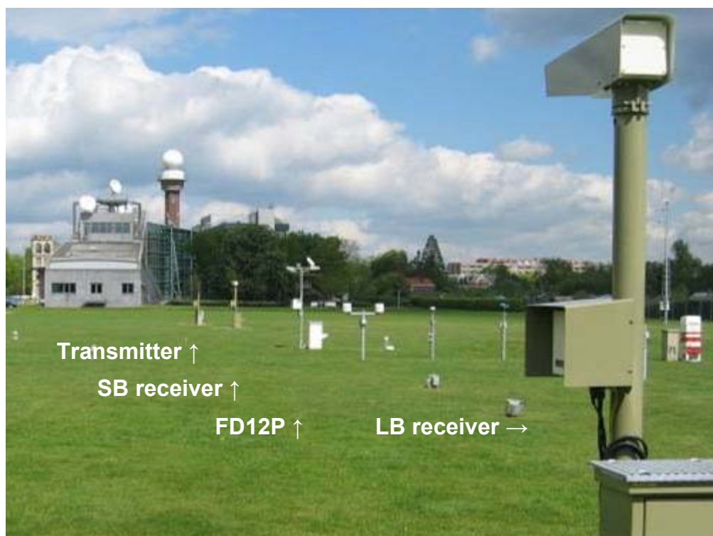
Figure 3: Setup for MOR calibration of the FD12P in De Bilt showing the transmitter and short baseline (SB) receiver of the TMM in the background (left), the reference FD12P in the middle, and the long baseline (LB) receiver of the TMM in the foreground (right).
