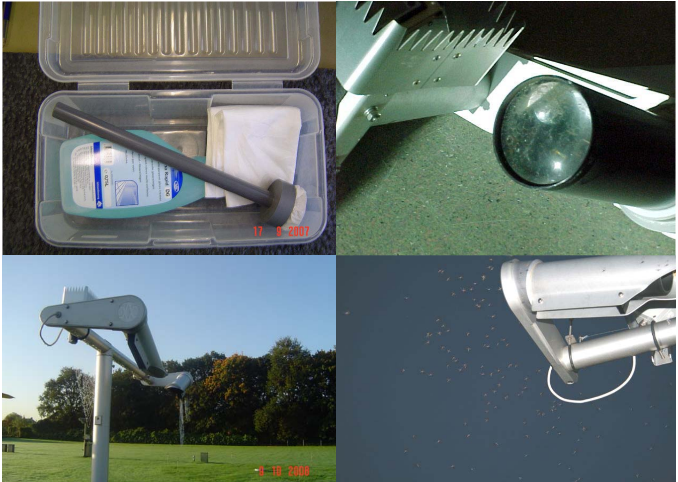
Figure 7: The FD12P cleaning kit (top left); an example of a contaminated lens of the FD12P resulting in an error status (top right); spider webs with dew on the FD12P (bottom left); and flying insects around the FD12P (bottom right panel).
