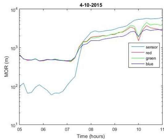
Figure 18: Graph of the estimated MOR(m) vs time (hours) for a foggy day. Plots of present weather
