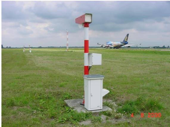
Figure 1: Transmissometer setup, consisting of a transmitter (Xenon flash lamp) and two receivers.
