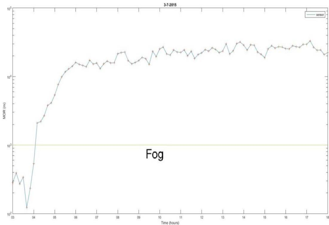
Figure 11: MOR of FS for July 3, 2015 a day with fog in the morning. The yellow line indicates the MOR upper limit for fog (1000 m).
