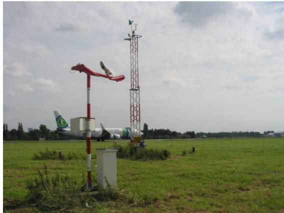
Figure 2: Forward scatter sensor (present weather sensor), which emits an infrared beam of light that is scattered into the receiver.
