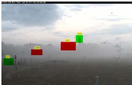
Figure 9: Fog covers objects at 108m and 170m. Closest and furthest object still visible. FS visibility = 122 m.
