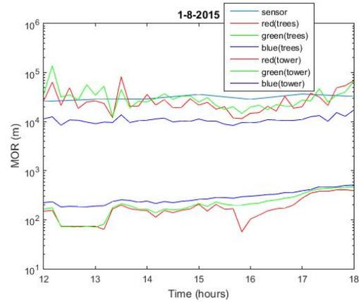
Figure 16: Graph of the estimated MOR(m) vs time(hours) for a clear day. Plots of present weather sensor data, MOR estimation from the 'trees' targets and from the 'tower' set of targets for the colour channels (RGB) are shown.
