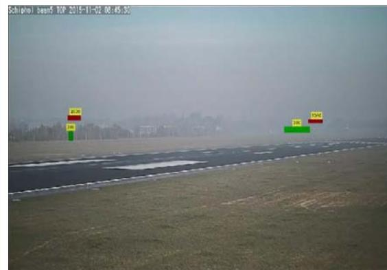
Figure 14: Hazy image of Schiphol 18R touchdown on the same day. The tree groups aren't detected anymore, while the left tree group is still visible to an observer.
