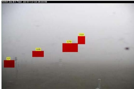
Figure 10: Fog covers almost the entire image. None of the landmarks are visible. PWS visibility = 61 m.
