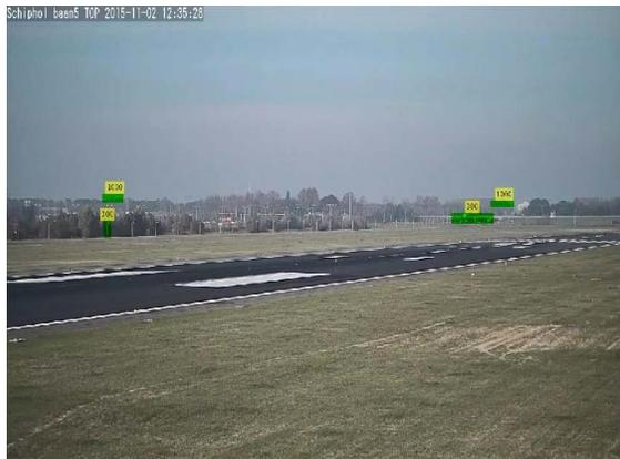
Figure 13: Clear image of Schiphol 18R touchdown. All landmarks (lamppost, viaduct both at 300 m, 2 tree groups at 1 km) are visible.
