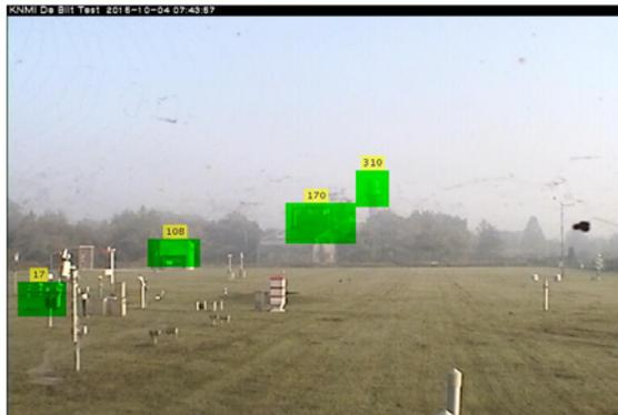
Figure 6: Image of a hazy day. All objects in the rectangles are visible (=green). FS visibility = 866 m.
