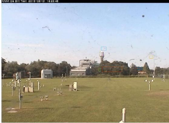
Figure 15: Input image of a clear day. Red, blue(front) and yellow rectangles indicate 'trees' set of targets used, while green, purple and blue(back) rectangles indicate the 'tower' set.
