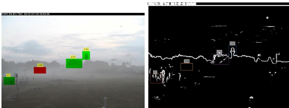
Figure 4 (left): Image obtained from the camera at the test field of KNMI. Figure 5 (right): Same image after edge detection is applied. The rectangles indicate the areas which were used for recognition of the object within them. The numbers above them indicate the distance in meters between the camera and the object in the rectangle.
