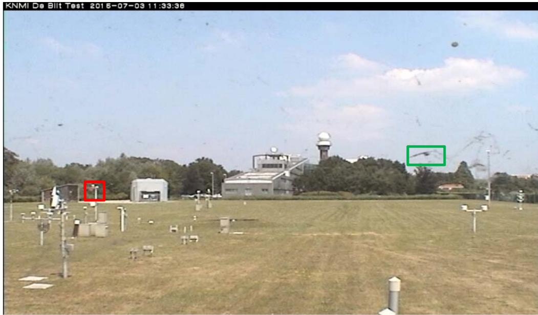
Figure 3: Example of an original image of the test field of KNMI on a clear day. Note the lens contamination (green) and the forward scatter visibility sensor (red).
