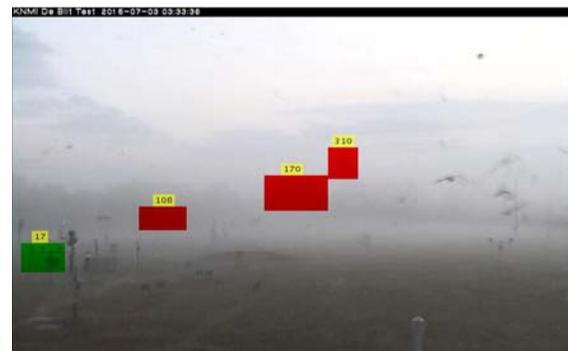
Figure 7: Foggy image. Only the closest landmark is visible, others aren't (=red). FS visibility = 339 m.
