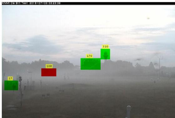
Figure 8: Ground fog. Only the object at 108m isn't visible. FS visibility = 272 m.
