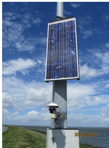
Figure 2.3: Ground measurement meter on Houtribdijk. A solar panel is placed vertically above the meter.
