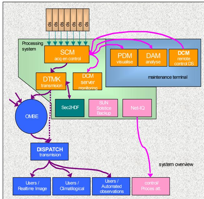
Figure 1. System overview software components
