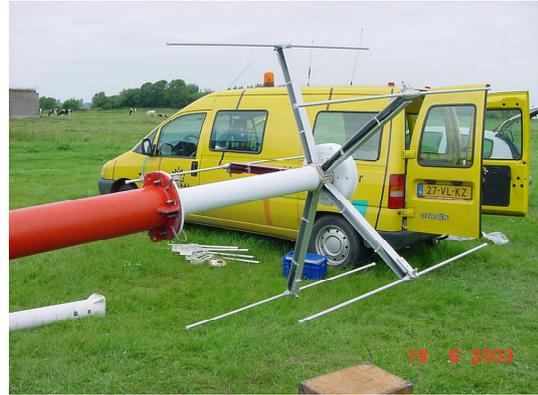
Figure 3. Top showing dipole-array and LF-antenna
