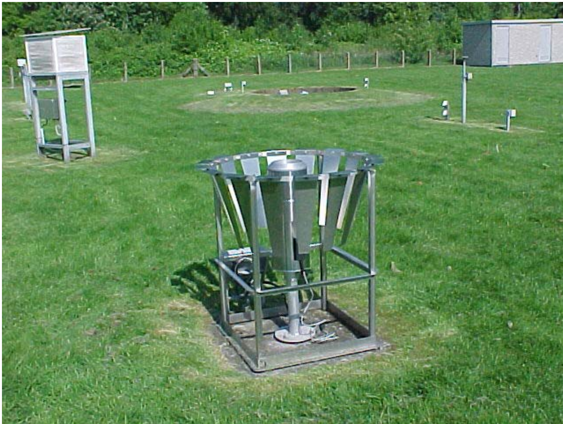
Figure 5: The Pluvio precipitation sensor on the measurement field during the field test in De Bilt. In the background the so-called English setup containing the operational KNMI precipitation gauge is visible to the North-Northwest.
