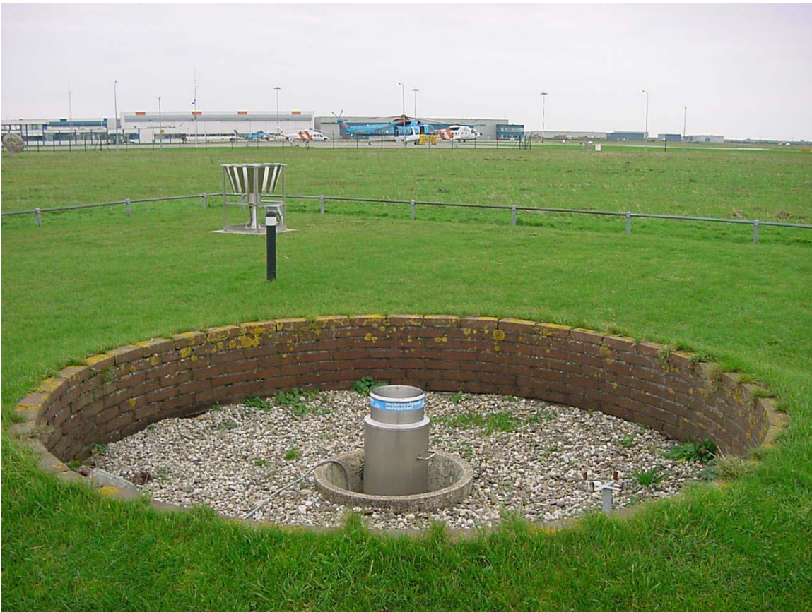
Figure 6: Picture of the Pluvio precipitation sensor on the measurement field during the field test in De Kooy. In the foreground the so-called English setup containing the operational KNMI precipitation gauge is visible and in the background the helicopter platforms and buildings to the South of the measurement field.
