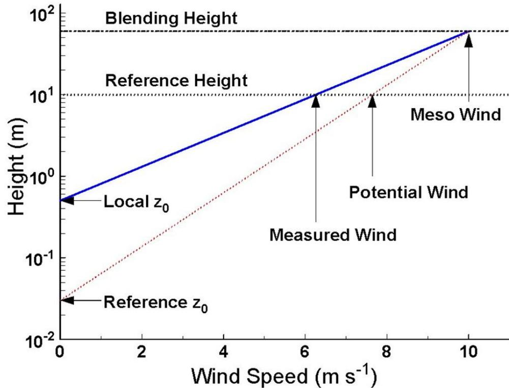
Figure 1: Schematic diagram explaining the concept of potential wind speed
