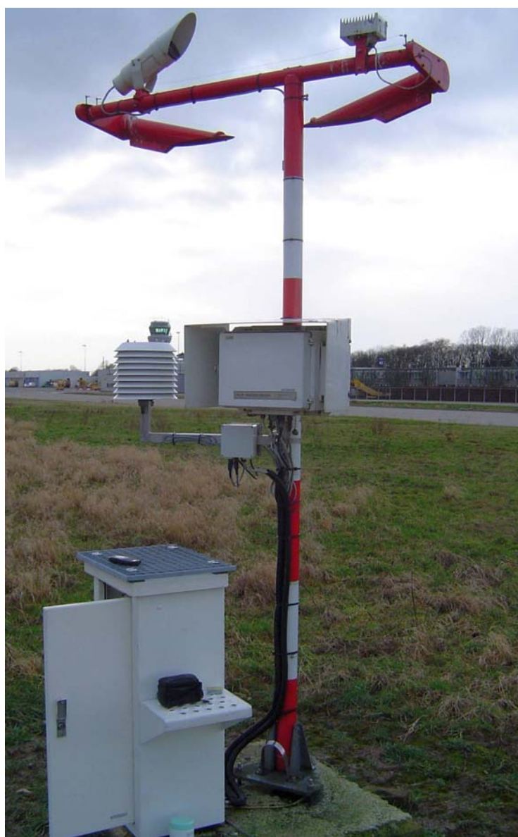
Figure 3. FD 1 2P at Maastricht Aachen Airport with the additional temperature and humidity sensor in the attached radiation screen.
