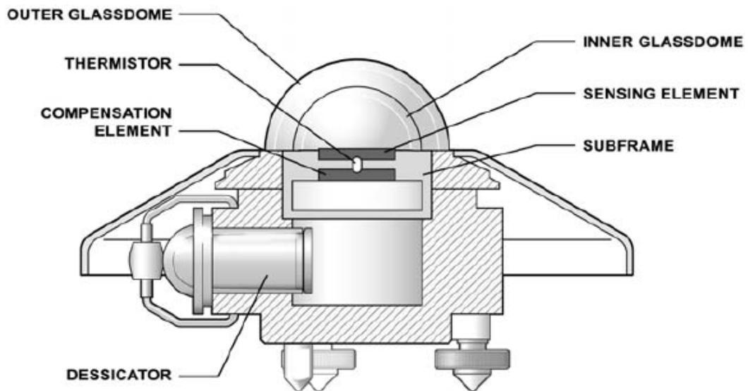
Figure 1.2: Drawing of Kipp&Zonen CM-11 pyranometer.
