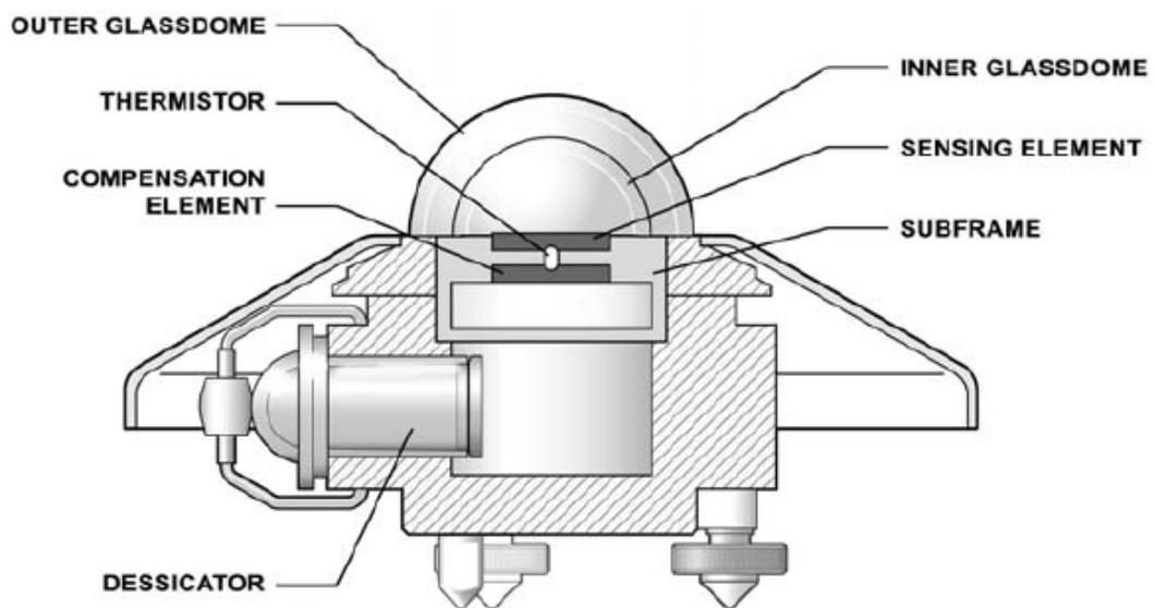
Figure 1.2: Drawing of Kipp&Zonen CM-11 pyranometer.
