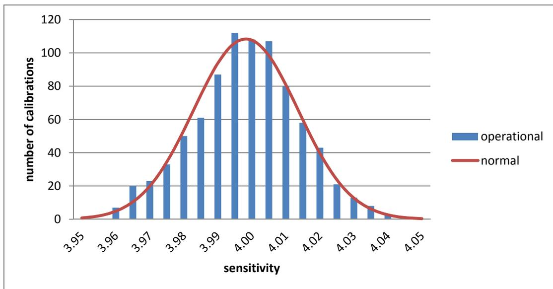
Figure 5.4: Histogram of operational calibrations without outliers compared to the normal distribution.
