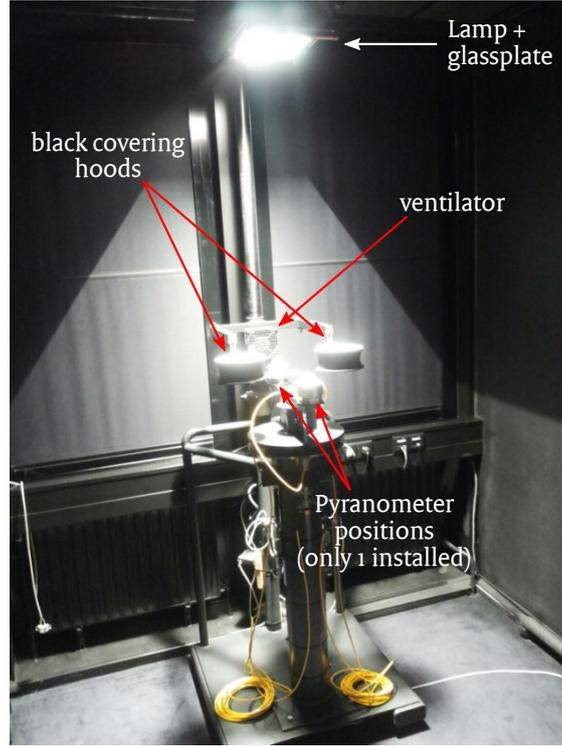
Figure 4.1: KNMI radiation calibration laboratory setup
