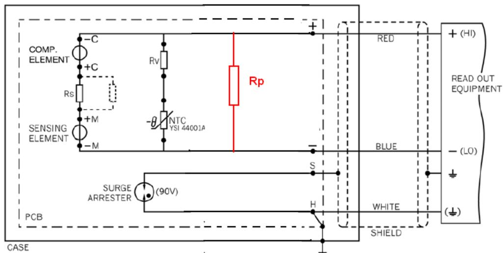
Figure 1.3: Schematics of the Kipp&Zonen CM-11 pyranometer.  $R_p$  is not present in a standard CM-11, but is added to provide a standardized sensitivity of  $4.00 \mu\text{V W}^{-1}\text{m}^2$ . To avoid affecting of the temperature compensation,  $R_v$  is increased to make sure that the decrease of the overall internal impedance of the sensor is compensated.
