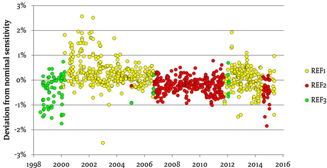
Figure 5.2: Calibration results of the KNMI network CM-11 pyranometers. The colour is determined by the reference sensor used in the calibration.
