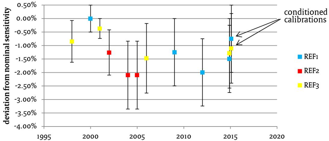
Figure 5.1: Deviation from original nominal sensitivity of the KNMI reference pyranometers found by PMOD-WRC in Davos for the period 1998-2015. All calibrations have been performed with unconditioned KNMI pyranometers, except in 2015, when REF1 and REF3 were each calibrated both conditioned and unconditioned.
