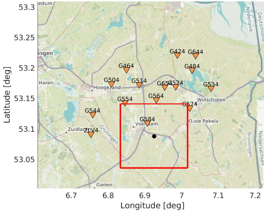
Figure 6: Overview map with locations of stations (yellow triangles) where P-wave onsets were picked, the fast Hypocenter solution (black dot) and the boundary line of the area in which a grid search is done (red box). Background map is from [www.openstreetmap.org](http://www.openstreetmap.org).
