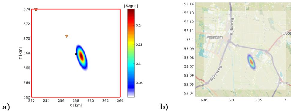
Figure 7: Maps showing the 95% confidence areas for (a) 1D and (b) 3D EDT (for a slice at 1000 m depth). (a) also depicts the initial Hypocenter solution (black dot) and the two nearest stations (orange triangles). (b) has, as a background, an Open Street Map of the Veendam Oude Pekela region. The white transparent region in (b) corresponds with the geographical area depicted in (a), (a) is in Rijksdriehoekstelsel whereas (b) is in wgs84.
