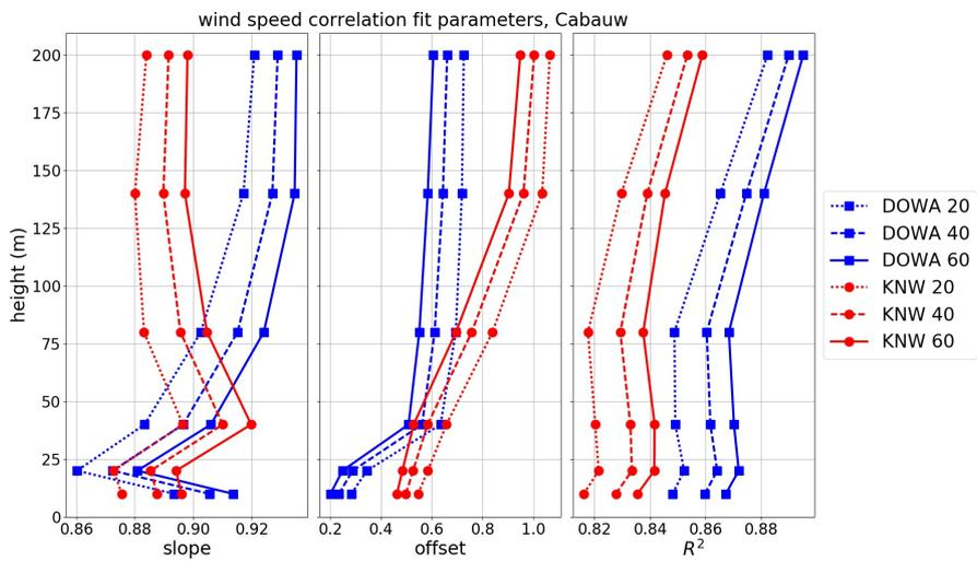
Figure 25: Height profile of the results of the linear regression (slope, offset and  $R^2$ ) of the wind speed data, comparing the DOWA (blue) and KNW atlas (red), for different averaging times (20, 40 and 60 minutes) of the mast measurements.
