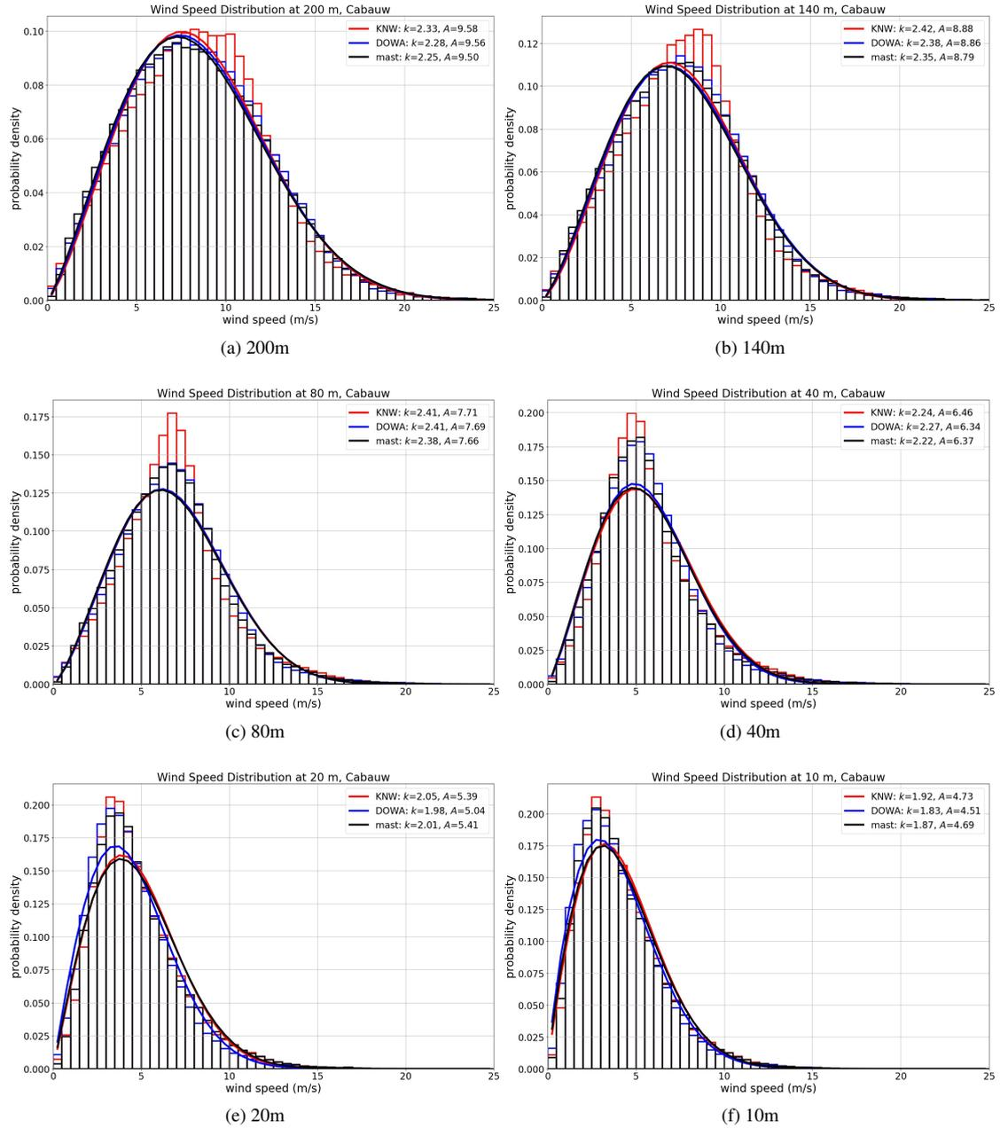
Figure 33: Wind speed distributions, with bin width of 0.5 m/s, showing mast measurements (black), DOWA (blue) and KNW (red) and corresponding Weibull fits (resulting fit parameters indicated in the legends).
