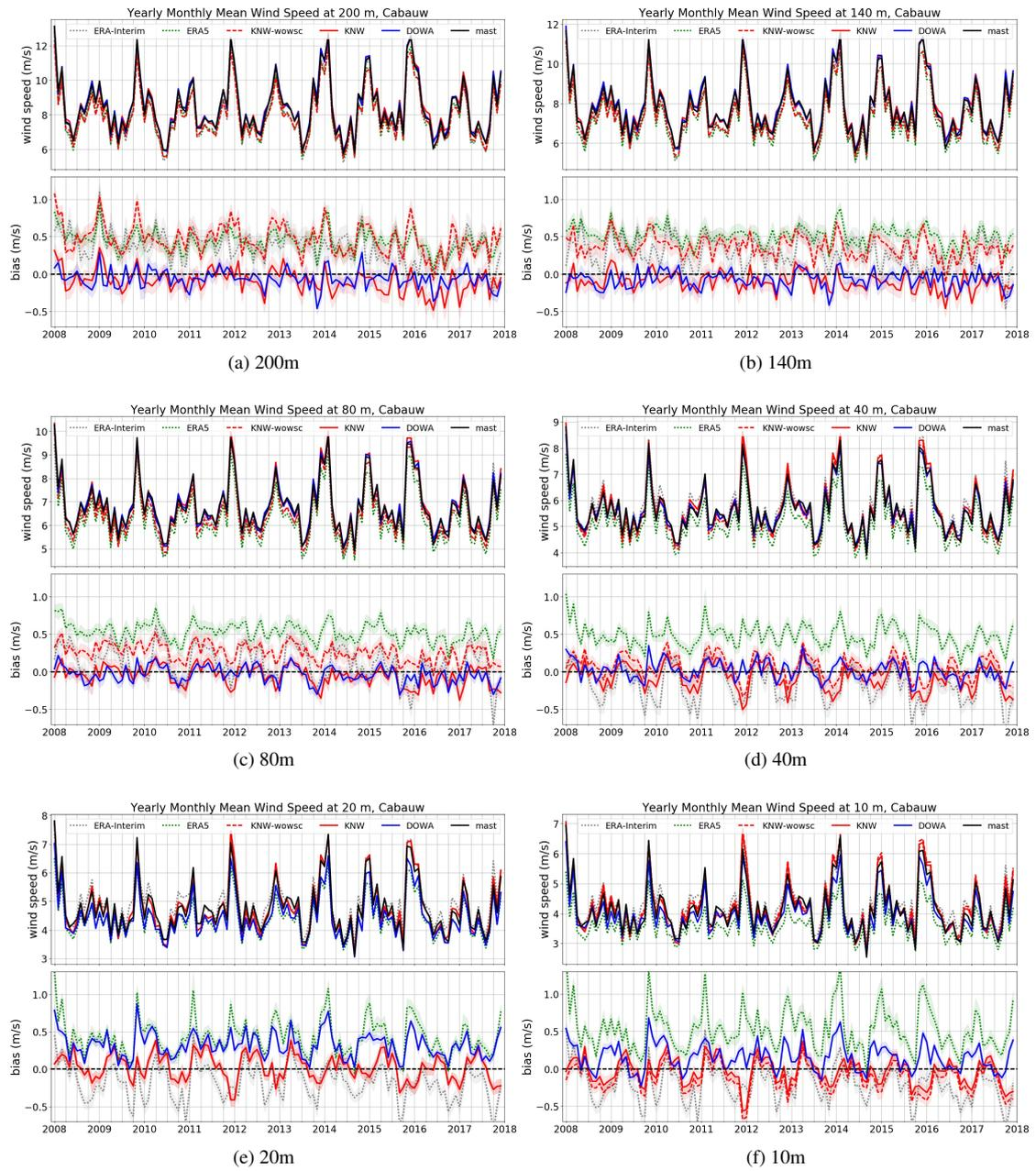
Figure 7: Yearly monthly mean wind speed, showing mast measurements (black), DOWA (blue), KNW atlas (red), KNW atlas without wind shear correction (red, dashed), ERA5 (green, dotted) and ERA-Interim (gray, dotted). Model variance is indicated by the shaded areas in the bias plots.
