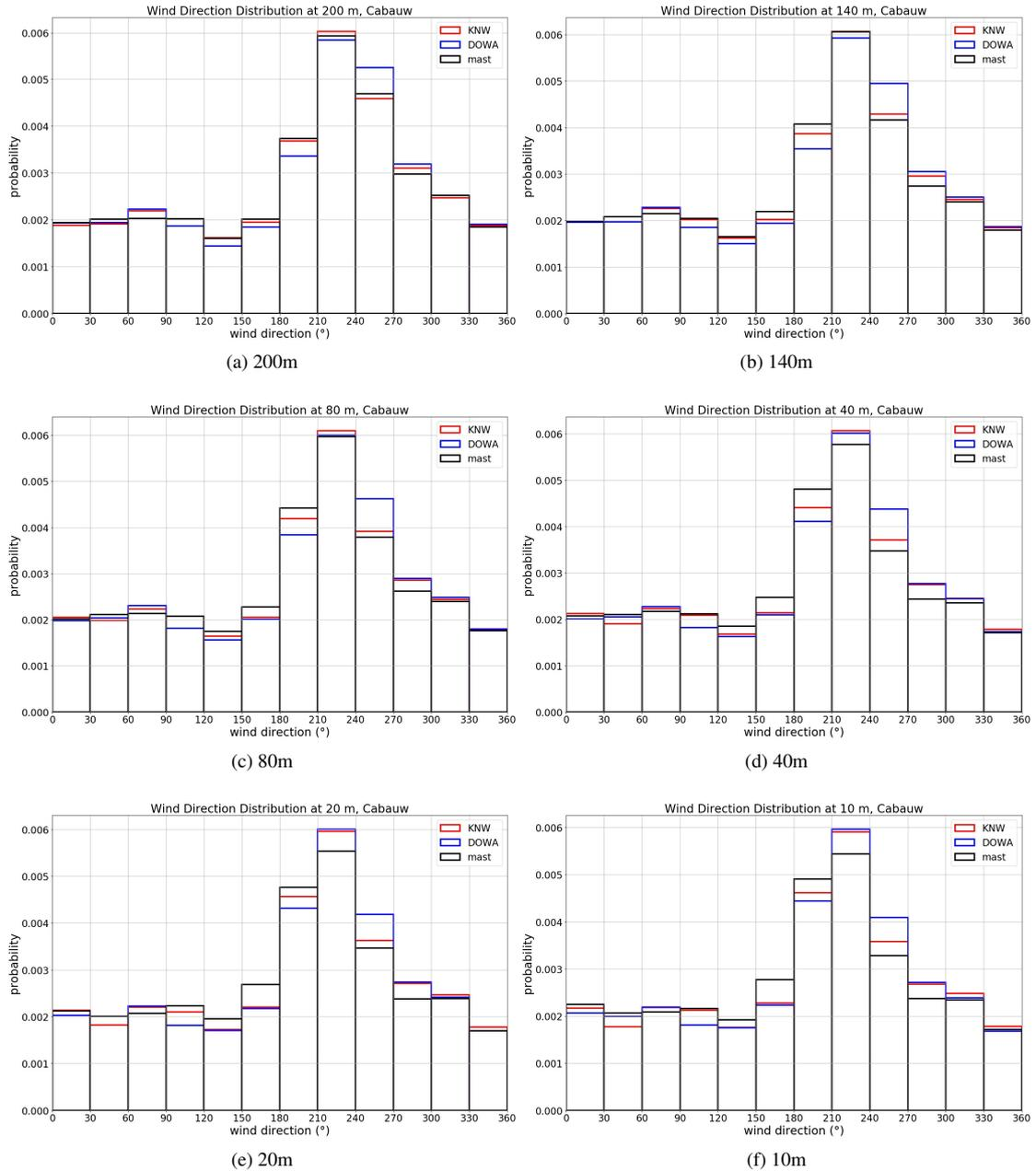
Figure 32: Wind direction distributions, with sector width of  $30^\circ$ , showing mast measurements (black), DOWA (blue) and KNW (red).
