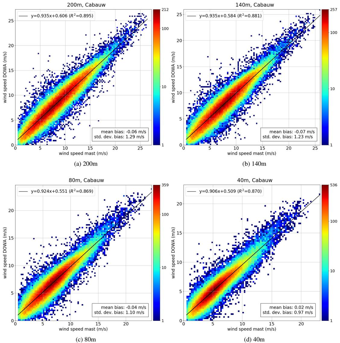
Figure 16: Scatterplot of the DOWA and mast wind speed data (visualized as a density plot with logarithmic color scale), showing the result of a linear regression (slope, intercept and  $R^2$ ) and the mean bias and standard deviation of the bias.
