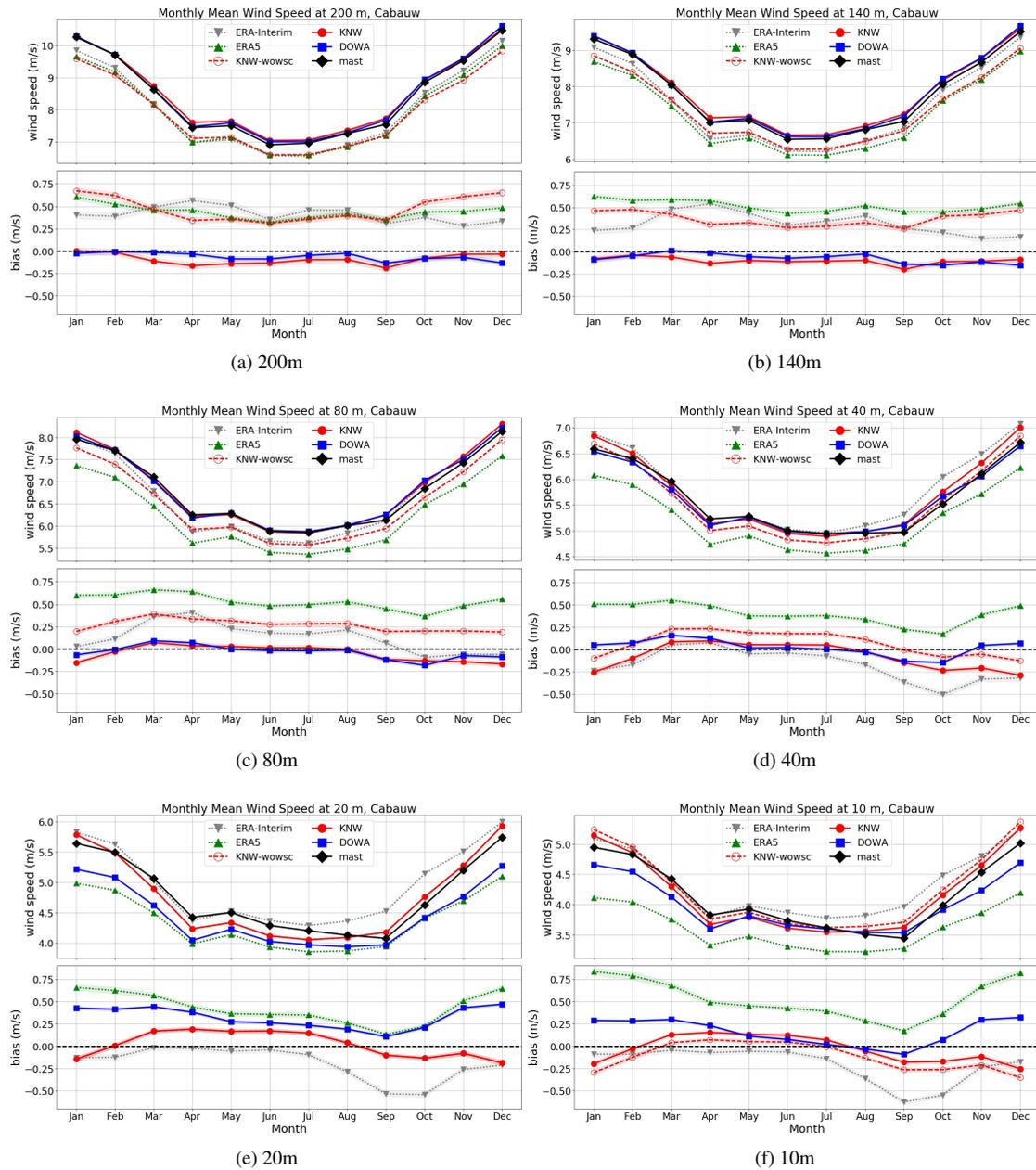
Figure 9: Monthly mean wind speed, showing mast measurements (black), DOWA (blue), KNW atlas (red), KNW atlas without wind shear correction (red, dashed), ERA5 (green, dotted) and ERA-Interim (gray, dotted). The upper panel shows the wind speed of both mast measurements and models, the lower panel the bias between the mast measurements and the models. Model variance is indicated by the shaded areas in the bias plots.
