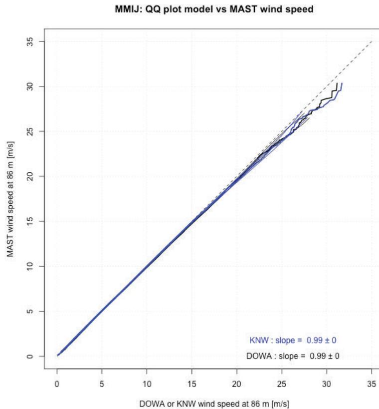
Figure 1: Quantile-quantile plots of wind speed data from two sources: mast vs. DOWA (black thick), and mast versus KNW (blue thick). Thin lines indicate the 90% compatibility interval. Text in plot gives slope estimates with their standard deviations.
