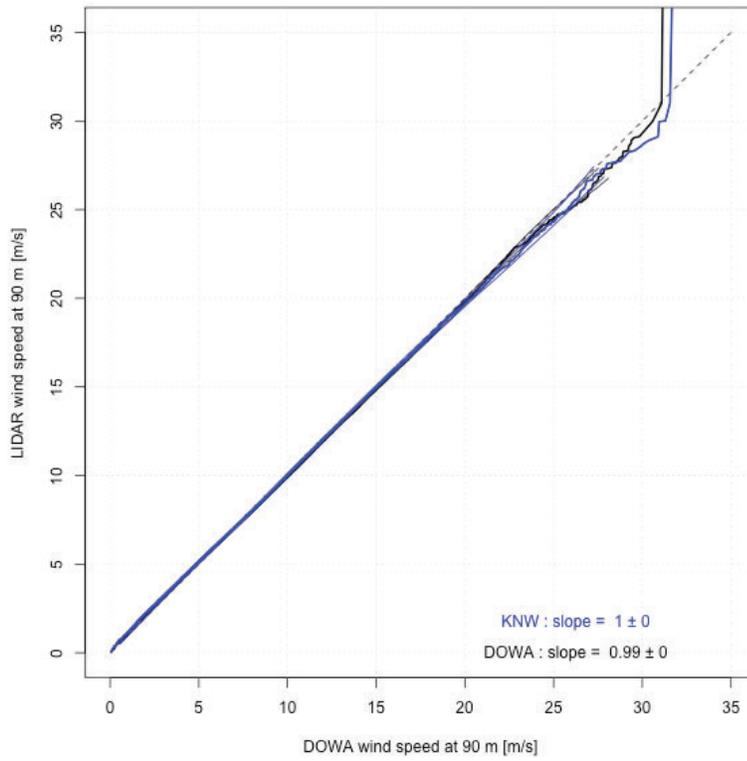
MMIJ: QQ plot MAST and LIDAR wind speed
