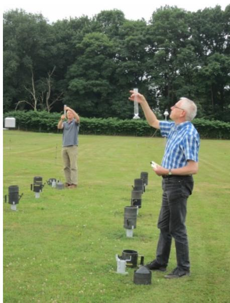
Photo 5: KNMI staff tapping the eleven manual rain gauges at 8:00 UTC.
