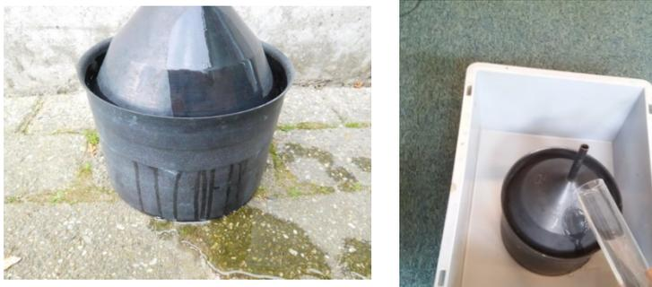
*Photo 3 Left: Rain gauge funnel turned upside-down, showing a (potentially) leaky rain gauge. Right: Performing the leakiness test. Note that water is added in the space between the funnel and the ring.*
