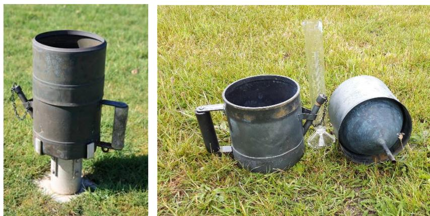
*Photo 1 Left: KNMI manual rain gauge (collecting surface 200 cm<sup>2</sup>) consisting of a reservoir (lower part) and a funnel (upper part). A ring with a height of 5 cm is attached to the funnel to clamp the funnel on the reservoir. The rim is at a height of 40 cm above ground level. Right: Funnel and reservoir taken apart and the measuring glass. Before each measurement the funnel is removed from the reservoir and the reservoir is emptied in the measuring glass.*
