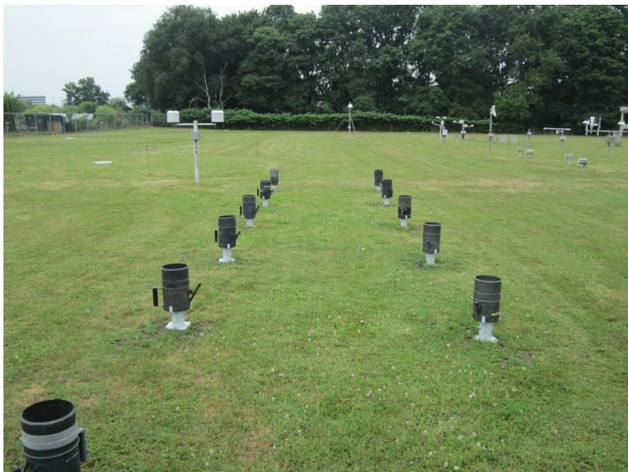
*Photo 4: Experiment at the KNMI test site in De Bilt comparing 11 manual rain gauges, performed in the period June 2017 – May 2018. Among the gauges are two old type gauges, four new type gauges, two new type gauges repaired with spot welding, two new type gauges with shifted rings, and a sealed new type gauge (lower left).*
