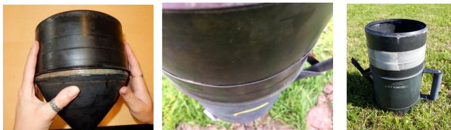
*Photo 2: From left to right: gauge with ring shifted upward, gauge repaired using spot welding but with gaps between the welding spots, and gauge sealed with special tape.*
