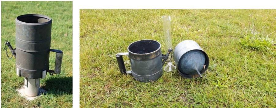
Figure 2.2: Left: KNMI manual rain gauge (collecting surface 200 cm<sup>2</sup>) consisting of a reservoir (lower part) and a funnel (upper part). Right: Funnel and reservoir taken apart and the measuring cylinder. Before each measurement the funnel is removed from the reservoir and the reservoir is emptied into the measuring cylinder.
