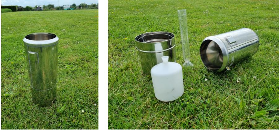
Figure 2.1: Left: Hellmann manual rain gauge (collecting surface 200 cm<sup>2</sup>) consisting of a reservoir (lower part) and a funnel (upper part). Right: Funnel and reservoir taken apart, the plastic container and the measuring cylinder. For the manual evaluation of the daily precipitation amount, the funnel is removed from the reservoir. Thereafter the container is emptied into the measuring cylinder.
