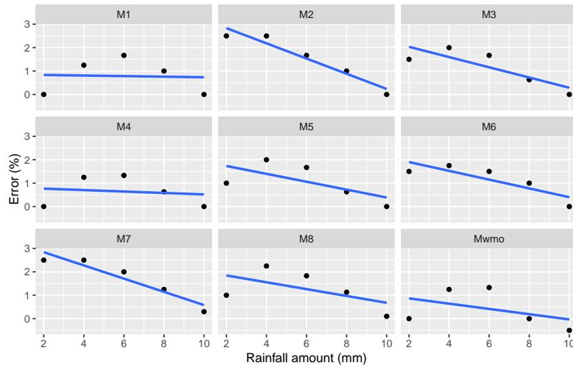
Figure A.1: Error resulting from the measuring cylinders as a function of rainfall amount in the cylinder. M1 corresponds to the measuring cylinder of R1, M2 of R2, etc. The straight line represents a linear regression fit.
