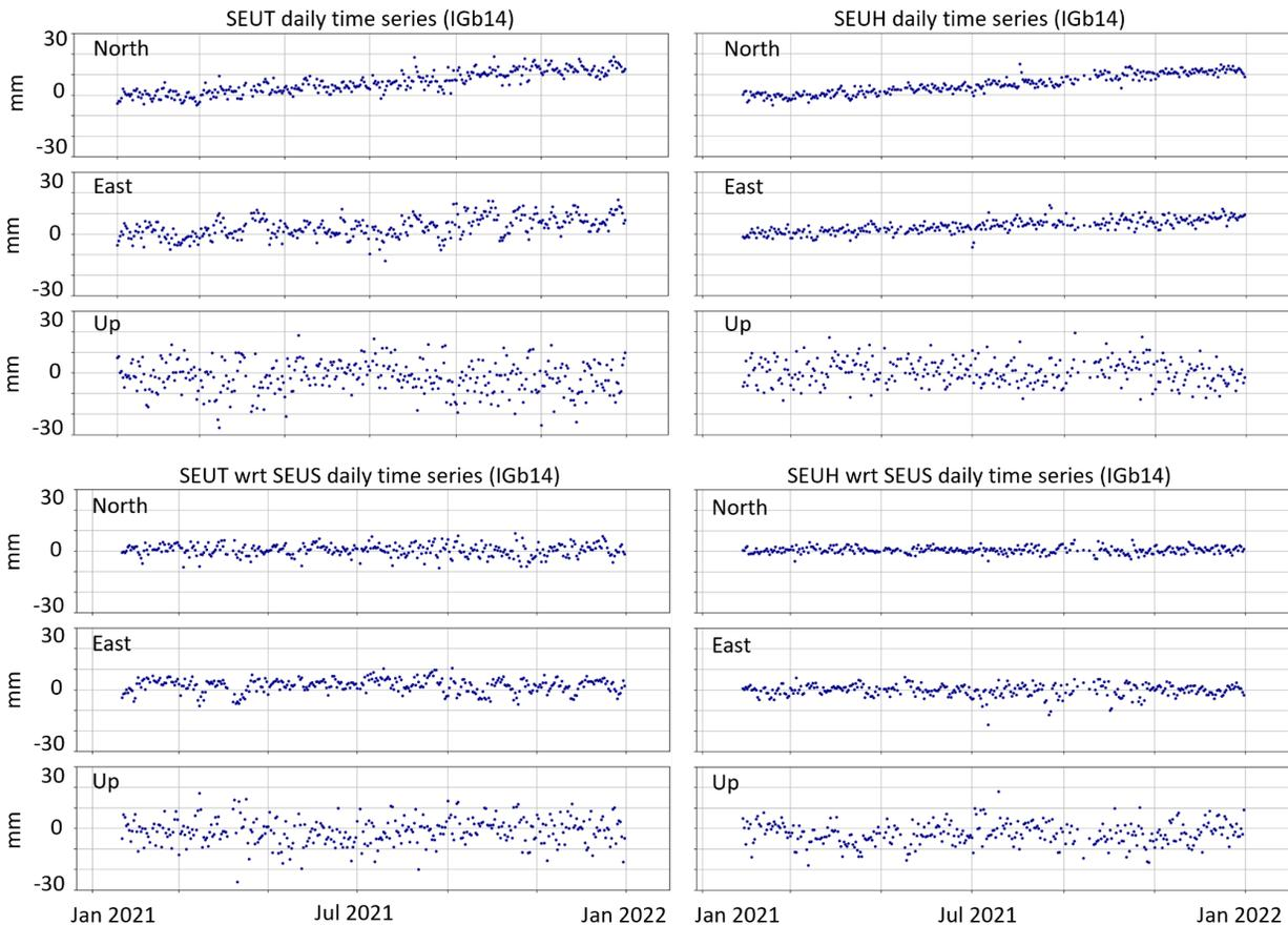
*Fig. 6: GNSS data from stations SEUT (upper left) and SEUH (upper right) from 2021. When the plate movement signal is removed, the data shows very little deviation from a horizontal line (bottom graphs SEUT and SEUH).*
