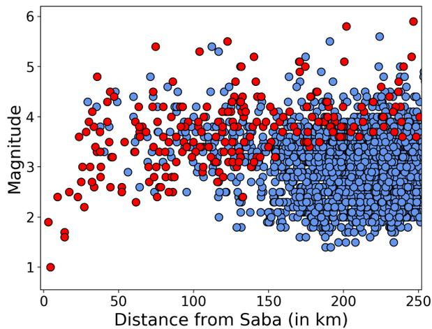
*Fig. 6: Magnitude-distance distribution of earthquakes located by KNMI (red) and reported by USGS (blue) in 2017-2021.*
