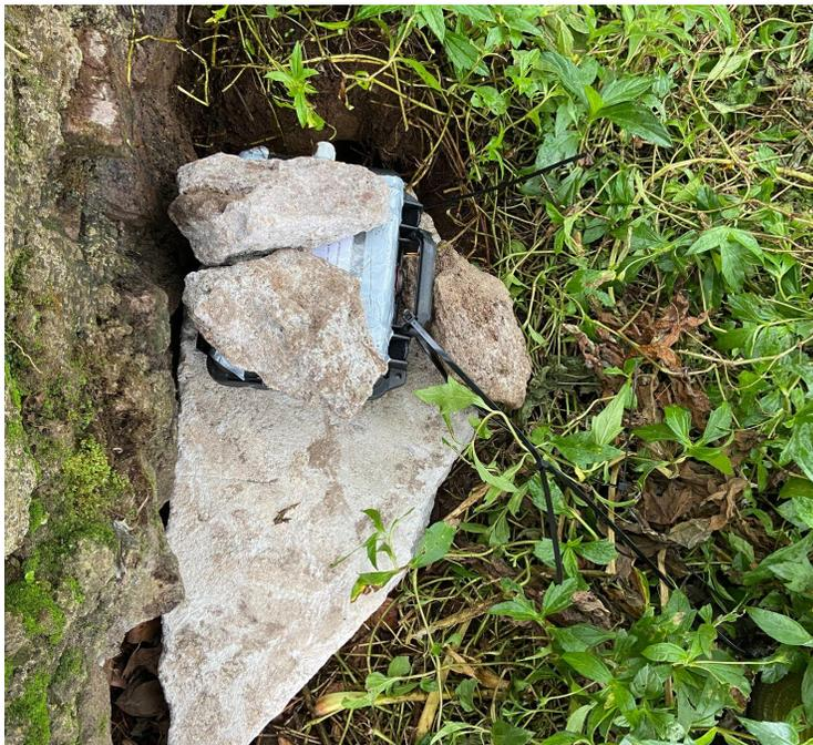
Fig. 13: Temperature sensor installed at the Green Gut. Data is stored locally and will be collected in 2023.
