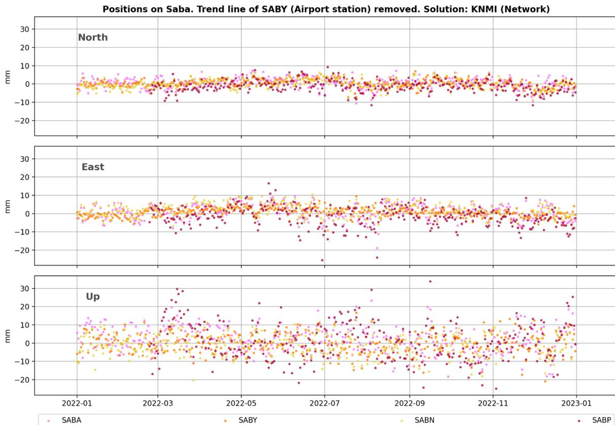
*Fig. 8: GNSS data from all permanent GNSS stations on Saba in 2022. The plate movement is removed from the signal. The data show very little deviation from a horizontal line.*
