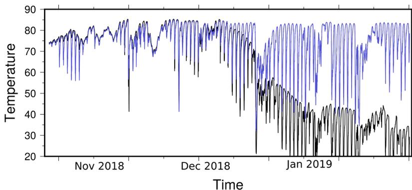
Figure 4: Recorded temperature (in degrees Celsius) at the hotspring opposite Green Island. Blue line depicts good data, black line shows compromised data quality with time due to failure of the temperature probe.
