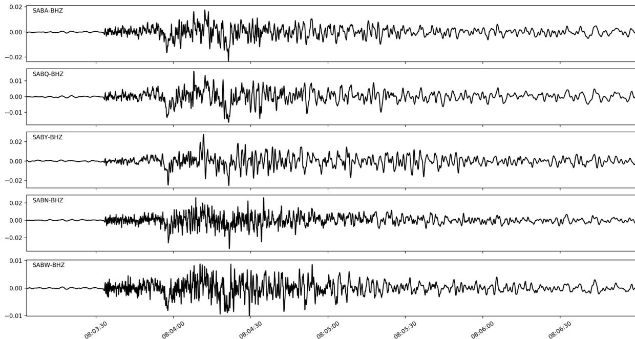
*Fig. 5: Recordings of the vertical ground displacement (in millimeter) caused by the M5.5 earthquake at 15-02-2022 08:03 UTC. This earthquake took place at a depth of about 50 km, about 240 km ESE of Saba.*
