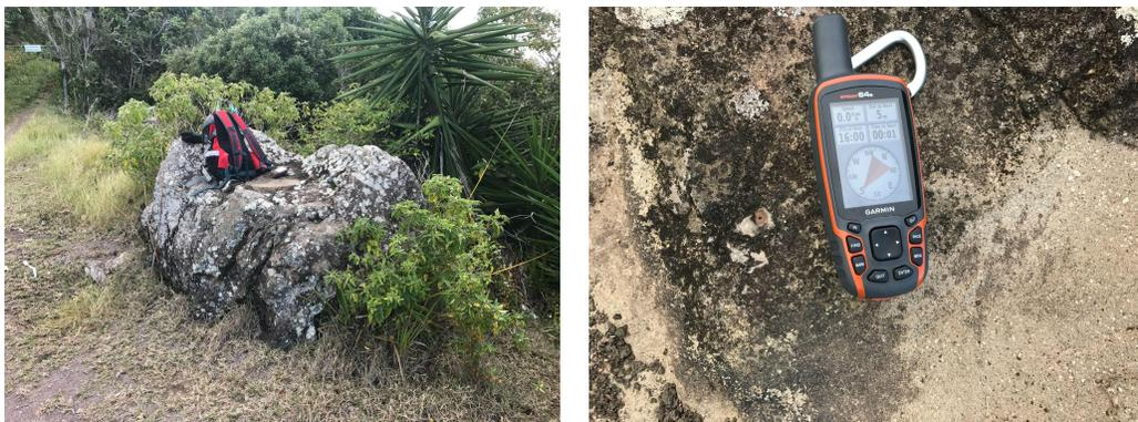
*Fig.9: The campaign gravity site Hells Gate. The marker that is measured is the tiny pin to the left of the handheld GPS.*
