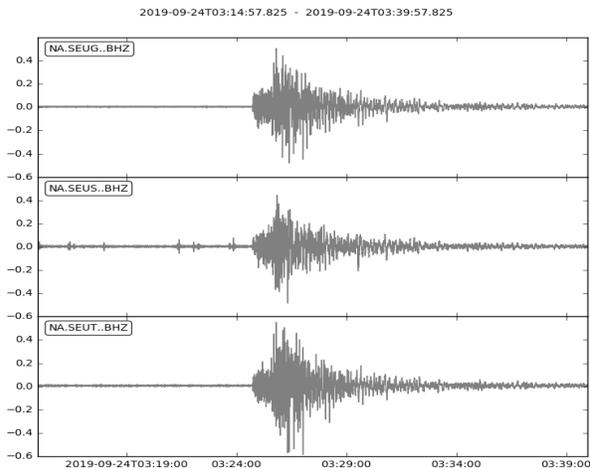
*Figure 2: Seismic recordings of the vertical ground velocity in mm/s measured by seismic stations SEUG, SEUT and SEUS due to an earthquake near Puerto Rico (source: USGS).*
