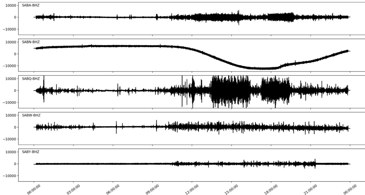
*Fig. 4: Vertical ground motion recorded by the seismic stations at Saba on 01-09-2021. Notice the increase of human induced seismic noise during the day, except at SABN. Here, however, a daily variation is clearly visible due to temperature variation. This is suppressed at the other stations by temperature regulation (air conditioning). Both the human induced noise and temperature variation do not limit the functioning of the seismometer and the detection of earthquakes.*
