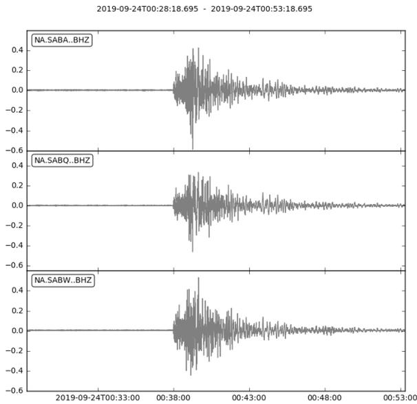
Figure 2: Seismic recordings of the vertical ground velocity in mm/s measured by seismic stations SABA, SABW and SABQ, due to an earthquake near Puerto Rico (source: USGS).
