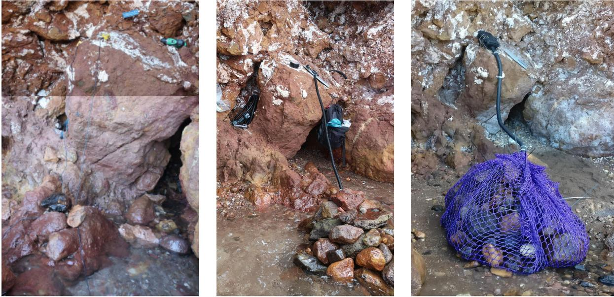
*Fig. 3 Temperature measurements of the hot spring opposite Green Island, in January 2018 (left), November 2018 (middle) and February 2019 (right). Temperature probes are buried in the ocean bed and covered with rocks to keep them in place. The data loggers are the small yellow cases mounted on the rock above the spring and housed in a black pelican case for additional protection from the elements in the most recent setup.*
