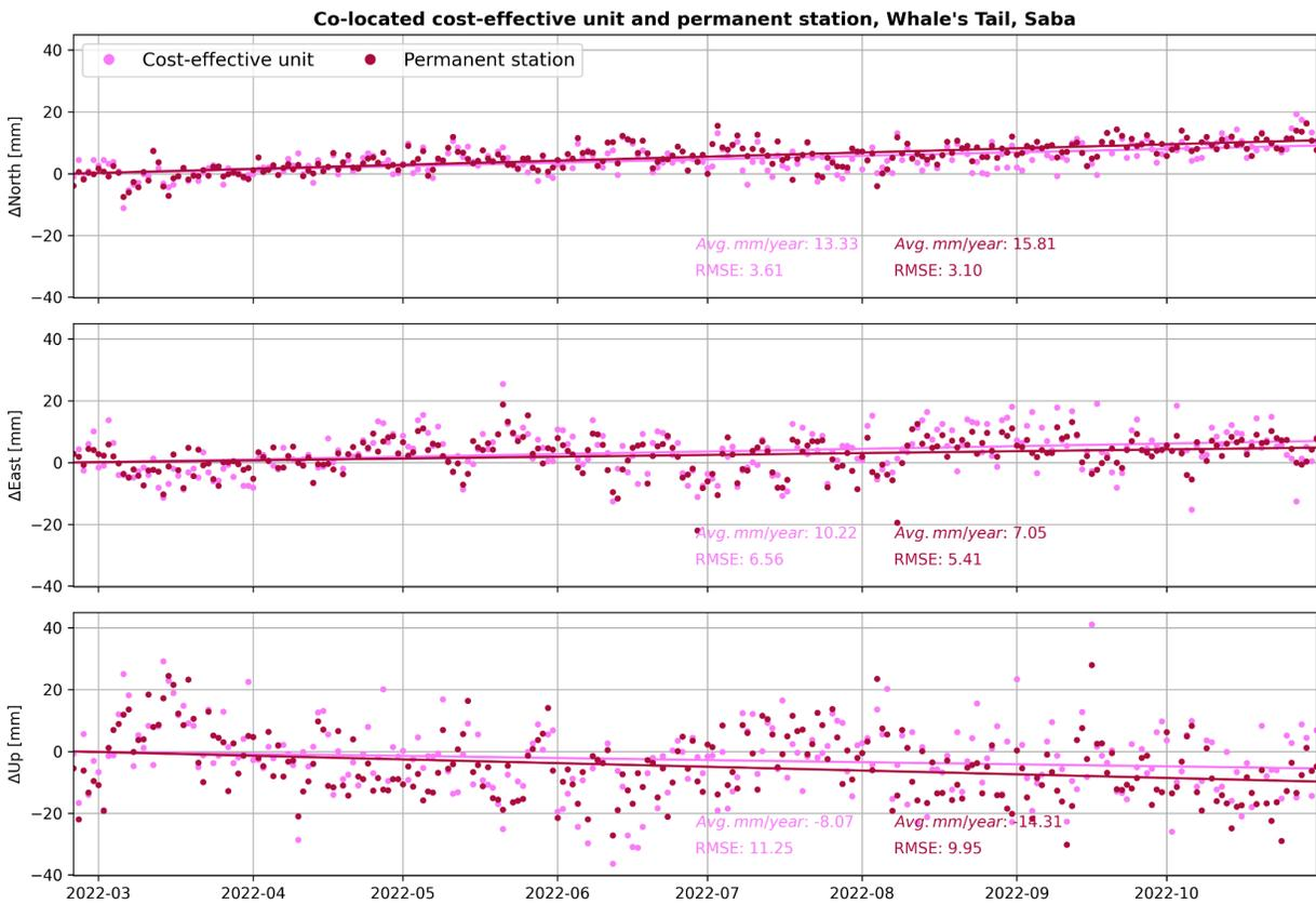
*Fig. 5 Daily positioning results in North, East and Up direction of the cost-effective unit and the permanent GNSS at the Whale's Tail over a time span of 8 months. The movements to the North and East are caused by plate tectonics and are visible in data from both instruments. The error (RMSE) in the vertical (up) direction is also comparable.*
