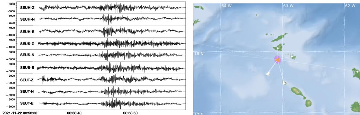
*Fig. 5: Seismic recordings (left) from the seismometers at St. Eustatius of an automatically detected earthquake in between St. Eustatius and St. Maarten (right). The earthquake took place on 22-11-2021, 08:58:20 UTC, at a depth of 76 km and has a magnitude of 2.7.*
