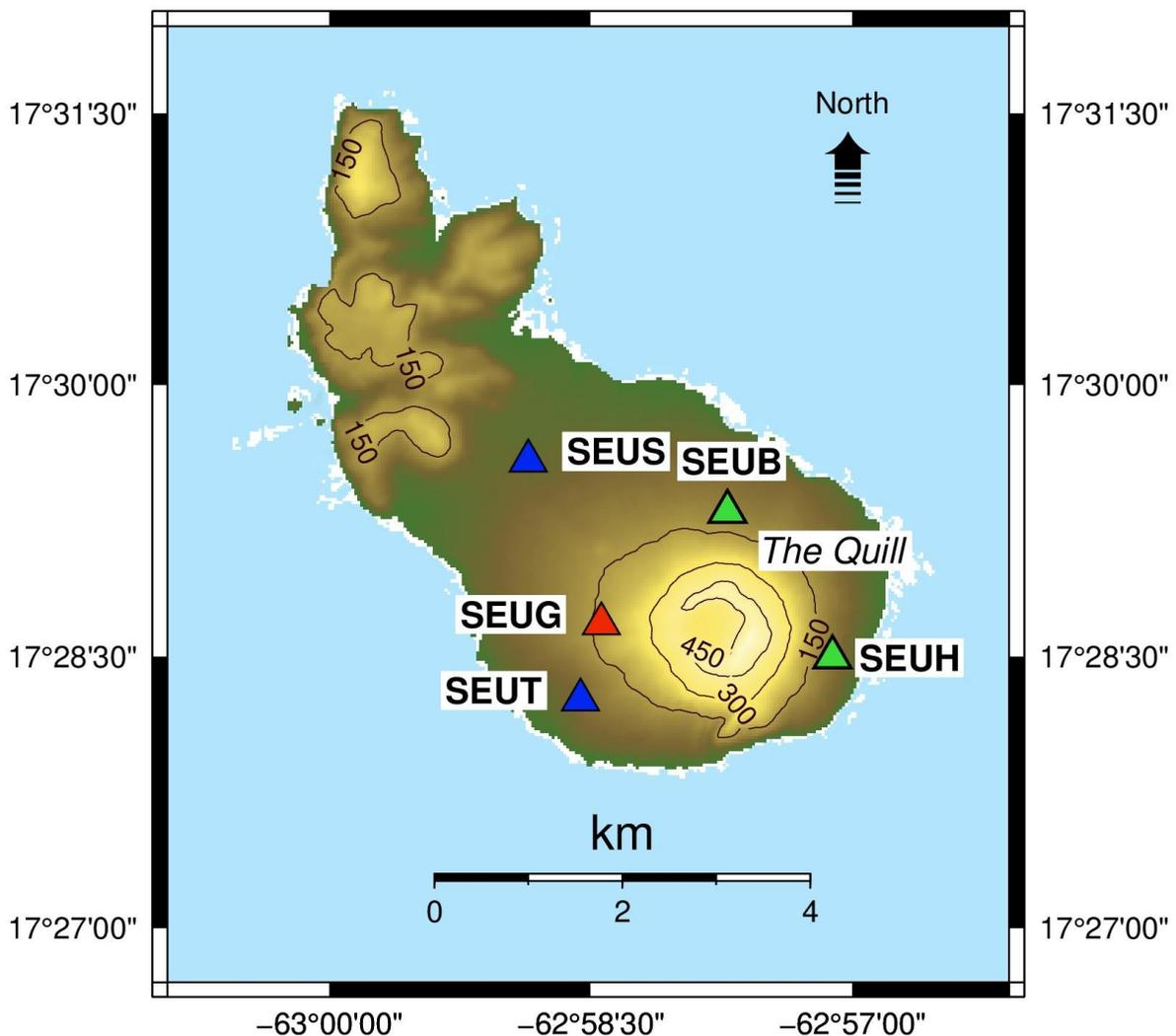
Fig. 1: Map showing the locations of current measurement sites on St. Eustatius with blue (GNSS/seismic stations) and red (seismic stations) triangles. GNSS/seismic stations that are self-sufficient are shown as green triangles.
