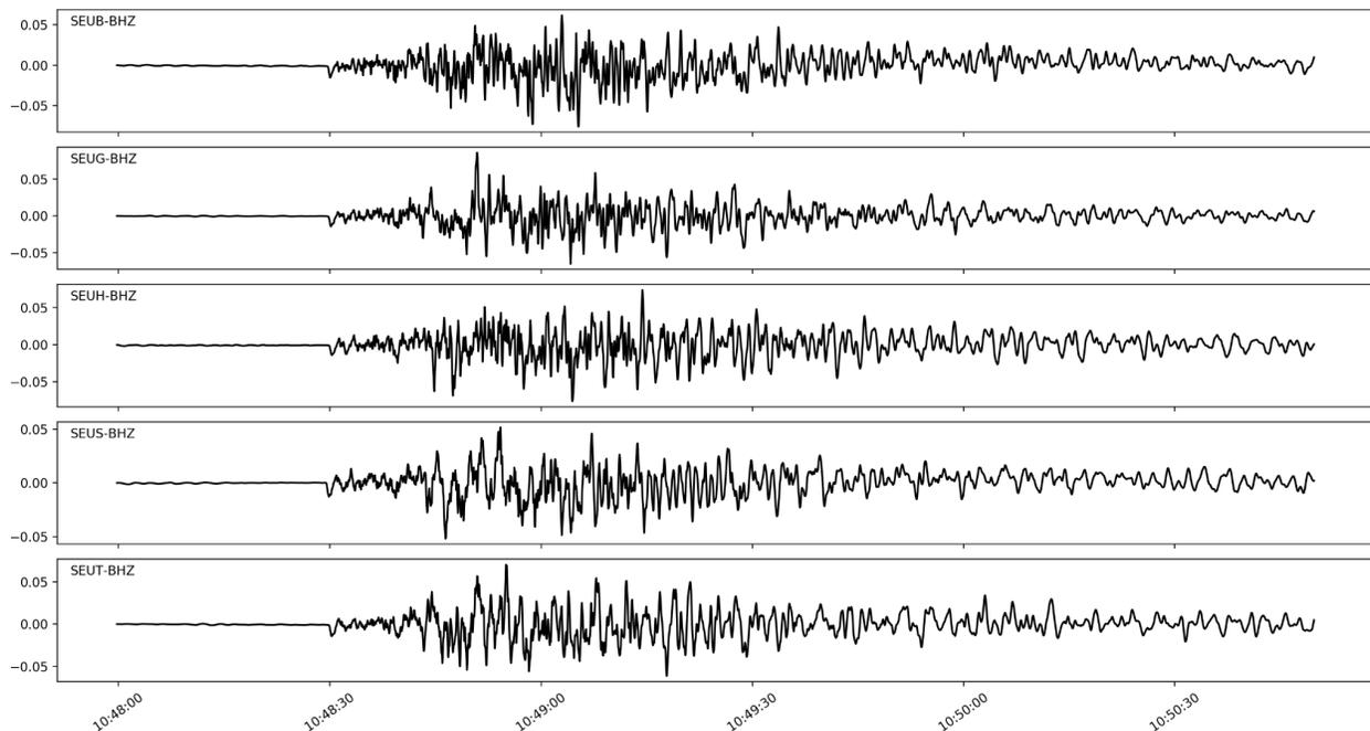
*Fig. 4: Recordings of the vertical ground displacement (in millimeter) caused by the M5.1 earthquake at 17-06-2022 10:48:12 UTC. This earthquake took place at a depth of about 40 km, about 100 km N of St. Eustatius.*
