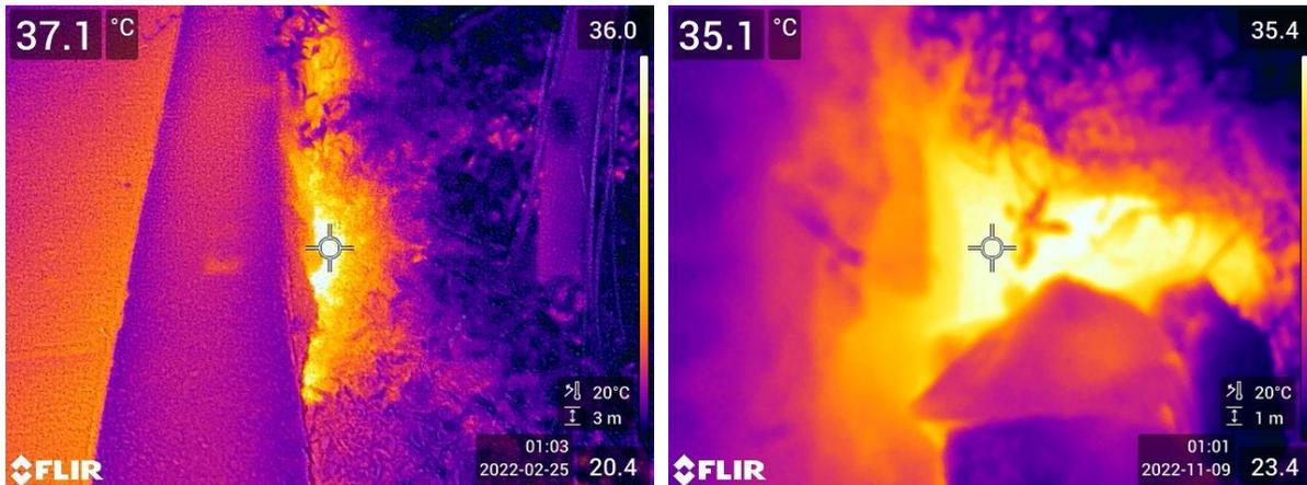
Fig. 12: Thermal camera images of the crack along the wall at the green gut measured in February 2022 (left) and November 2022 (right).
