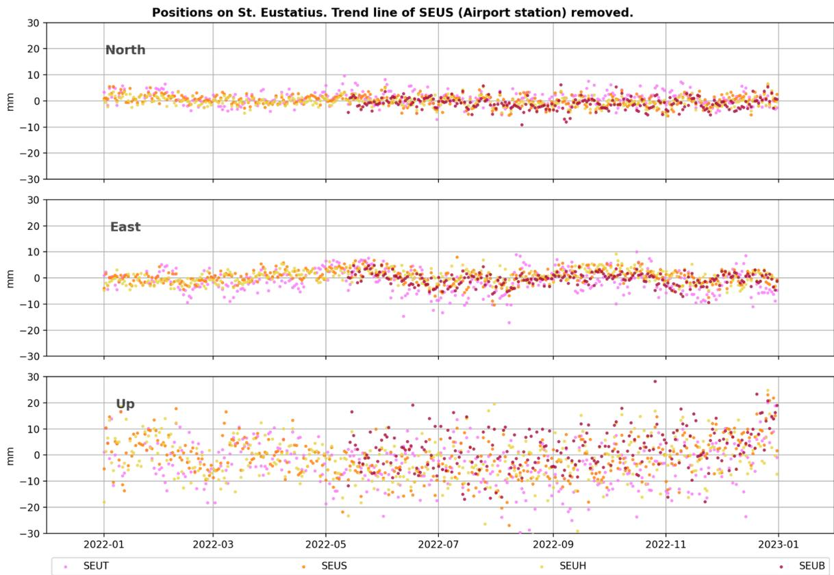
*Fig. 5 GNSS data from all permanent GNSS stations on St. Eustatius in 2022. The plate movement is removed from the signal. The data show very little deviation from a horizontal line.*
