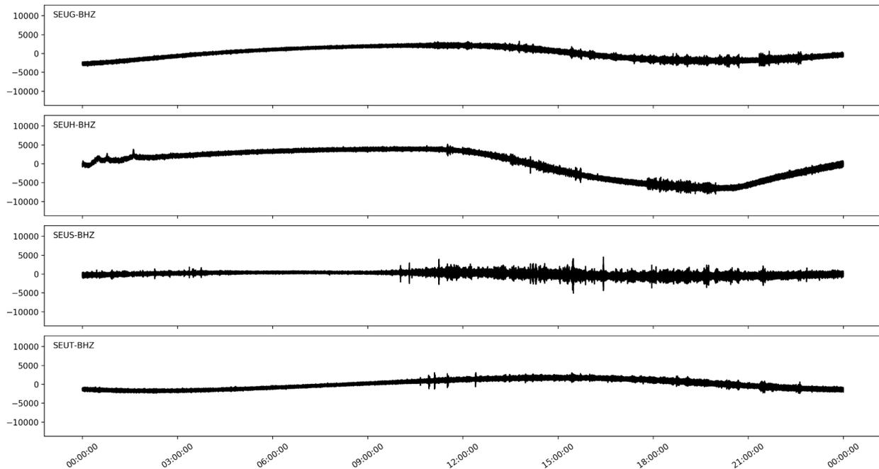
*Fig. 4: Vertical ground motion recorded by the seismic stations at St. Eustatius on 01-09-2021. Notice the increase of human induced seismic noise during the day at SEUS due to its vicinity to traffic and offices. A daily variation, which is most likely due to temperature variation, is visible in SEUG and SEUH, and less pronounced in SEUT. Both the human induced noise and temperature variation do not limit the functioning of the seismometer and the detection of earthquakes.*
