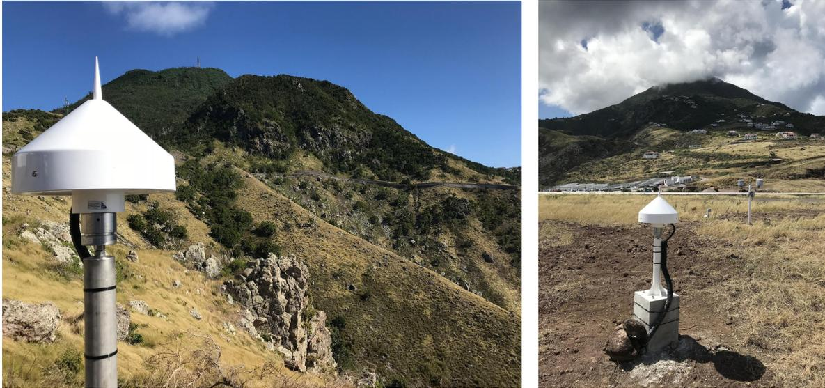
*Fig. 1 GNSS installation by St. Johns (left) and at the airport (right). The white part at the top is the antenna which receives the signals from satellites orbiting the Earth.*
