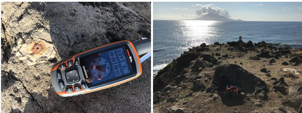
*Fig. 6: The campaign gravity site Hells Gate. The marker that is measured is the tiny pin to the left of the handheld GPS.*
