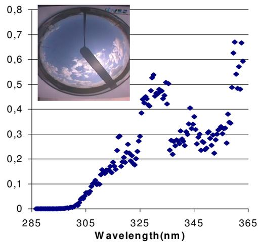
**Figure 3.1b.** UV-spectrum of a partial cloudy situation (Paramaribo, January 13 2003, 14:16 UTC; SZA is 35.3°), together with a picture from the Total Sky Imager of the same time. Between 320 nm and 360 nm some clouds 'pass' the sun.
