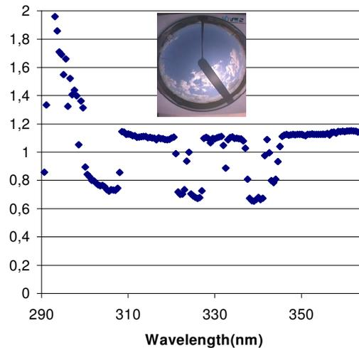
**Figure 3.2b.** UV-spectrum divided by the UV-spectrum of the reference (22 August 2003, 13:19 UTC; SZA is 35.3°) for the partial cloudy situation (Paramaribo, January 13 2003, 14:16 UTC; SZA is). The line is only smooth at sunny moments.
