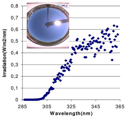
**Figure 3.1a.** UV-spectrum (measured by the Brewer) of a cloudless situation (Paramaribo, August 22 2003, 13:19 UTC; SZA is 35.7°), together with a picture from the Total Sky Imager of the same time. This spectrum is used as reference spectrum in selection 2, for the SZA range 35-36°.
