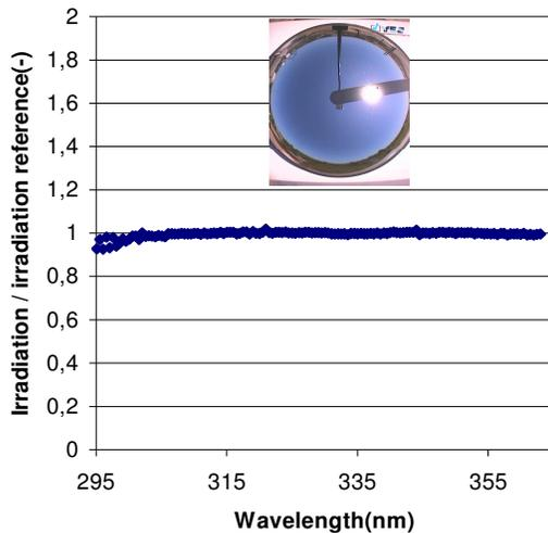
**Figure 3.2a.** UV-spectrum divided by the UV-spectrum of the reference (22 August 2003, 13:19 UTC; SZA is 35.7°) for a cloudless situation (Paramaribo, August 25 2003, 13:19 UTC; SZA is 35.4°). The line is almost smooth.
