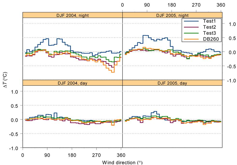
Figure 3.16: Daytime and nighttime temperature differences  $\Delta T$  between SiteX and Test4 as a function of wind direction ( $10^\circ$  bin width) for (a) winter (DJF) of 2004 (left panels), (b) winter (DJF) of 2005 (right panels). The second period represents the period after the renovation of the wasteland area.
