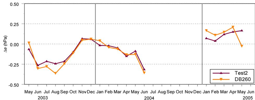
Figure 3.20: Monthly means of the daily vapor pressure differences  $\Delta e = e(\text{siteX}) - e(\text{Test4})$  for the period May 2003-June 2005. Missing month are due to malfunctioning of some of the relative humidity sensors.
