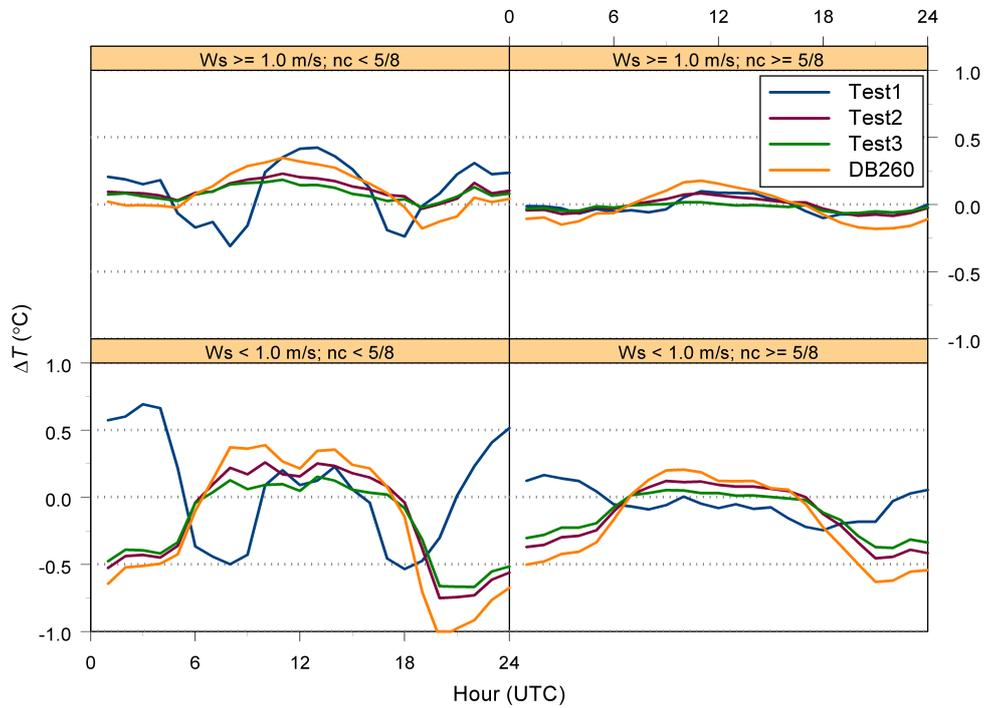
Figure 3.12: Diurnal cycles of the mean temperature differences between SiteX and Test4 for the summers (JJA) of 2003 and 2004 (before the renovation of the wasteland area) for four combinations of wind speed  $W_s$  and cloud cover  $nc$  (fraction of cloud cover) as indicated on top of each panel. The 10-min values are grouped together in 24 hourly values.
