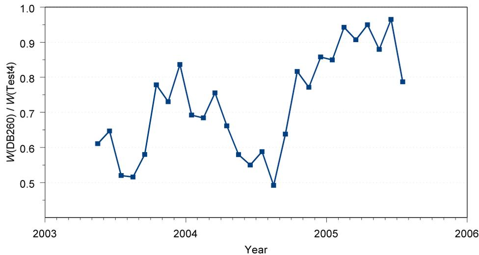
Figure 3.15: Monthly mean wind speed DB260, expressed as a fraction of the monthly mean wind speed at Test4 for small 10-min wind speeds ( $W_{s,Test4} \leq 1.0$  m/s) for the period May 2003-June 2005.
