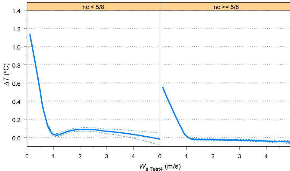
Figure 3.13: Relationship between the nighttime temperature differences between Test1 and Test4 and 1.5 m wind speed ( $W_s$ ) at the Test4 site for two categories of cloud cover  $nc$  (fraction of cloud cover). Values refer to the May 2003 – June 2005 period. The solid lines are locally weighted running line smooth curves (Cleveland, 1979) with a span of 0.5. The dashed curves give the point-wise 2 times standard-error bands.
