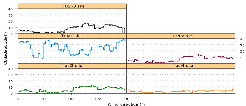
Figure 2.1: Obstacle altitude as a function of wind direction at DB260 and the 4 parallel sites.
