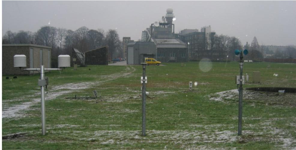
*Figure 2.5: Instruments at DB260. The left side shows the KNMI multi-plate radiation shields for measuring temperature and relative humidity. The right side shows the cup anemometer. Both instruments operate at 1.5 m above ground level. The 4 parallel sites are equipped with the same instruments and have an identical set-up.*
