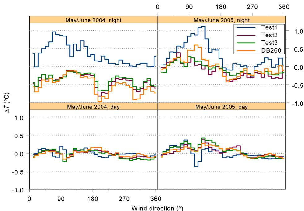
Figure 3.17: Daytime and nighttime temperature differences  $\Delta T$  between SiteX and Test4 as a function of wind direction ( $10^\circ$  bin width) for (a) May/June 2004 (left panels), (b) May/June of 2005 (right panels). The second period represents the period after the renovation of the wasteland area.
