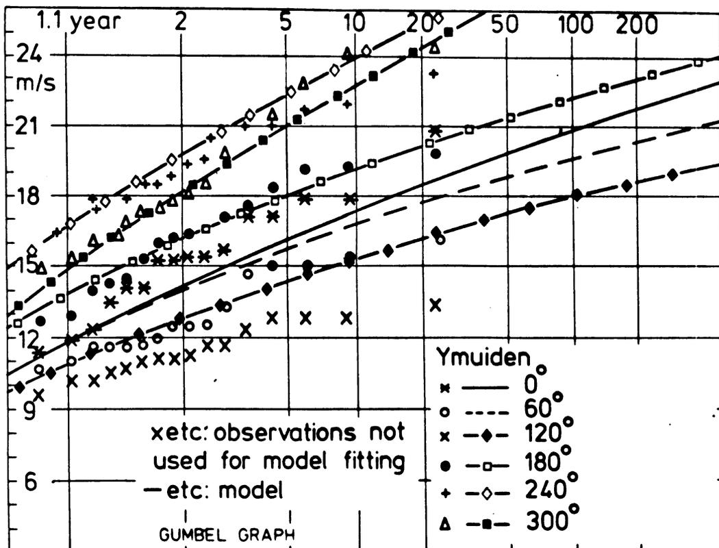
Fig. 20.14 Annual azimuth-sector maximum hourly wind speed for IJmuiden as observed and as computed from the model independent of these observations.
