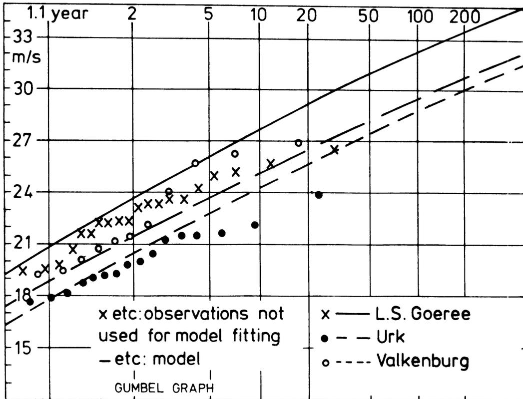
Fig. 20.5 Annual maximum hourly wind speed for Lightvessel Goeree, Urk and Valkenburg as observed and as computed from the model independent of these observations.
