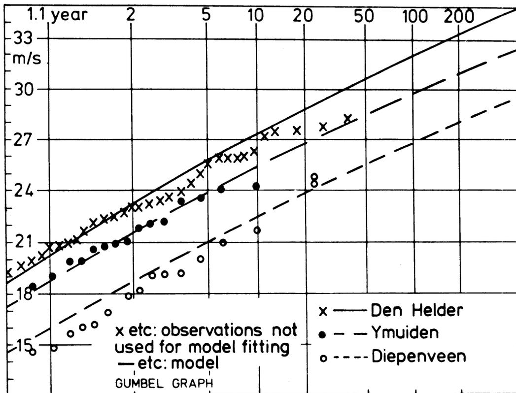
Fig. 20.1 Annual maximum hourly wind speed for Den Helder, IJmuiden and Diepenveen as observed and as computed from the model independent of these observations.
