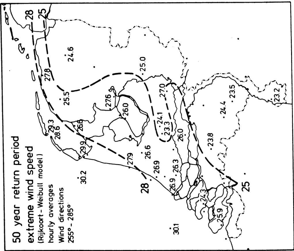
Fig. 24.10 Extreme values of hourly average wind from the 270° azimuth sector with mean recurrence time of 50 years, computed for all stations from the compound model.
