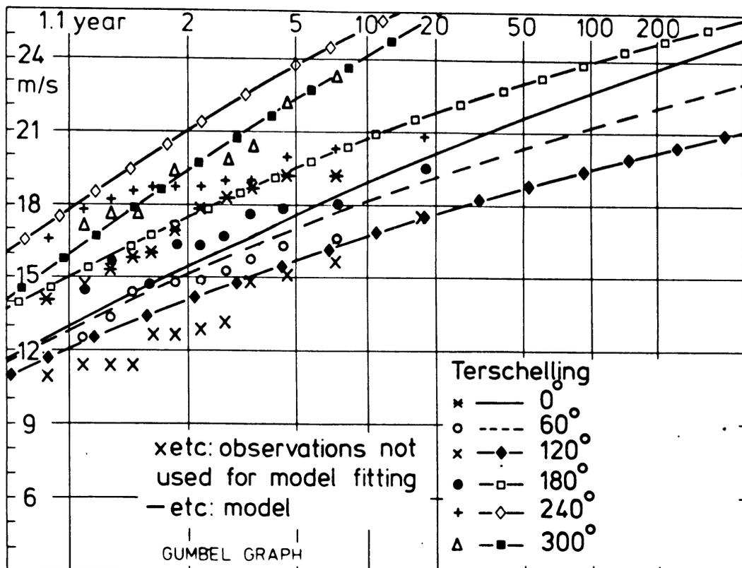
Fig. 20.12 Annual azimuth-sector maximum hourly wind speed for Terschelling as observed and as computed from the model independent of these observations.
