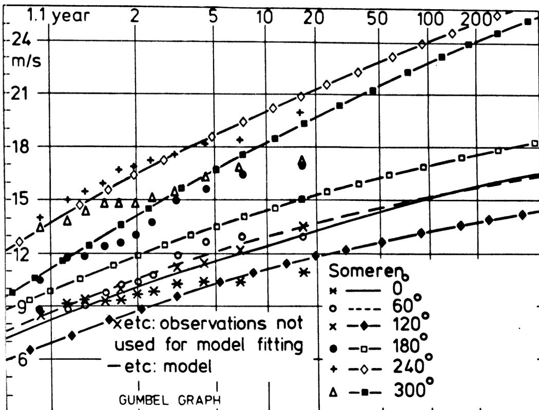
Fig. 20.16 Annual azimuth-sector maximum hourly wind speed for Someren as observed and as computed from the model independent of these observations.
