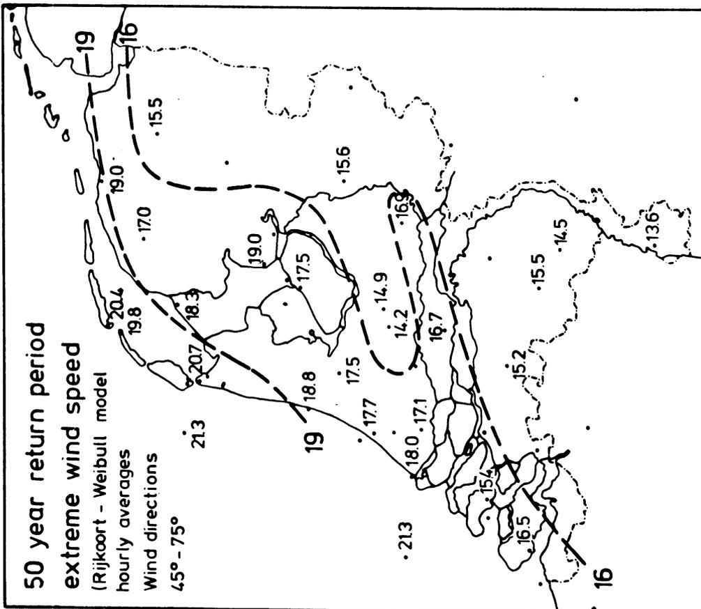
Fig. 24.3 Extreme values of hourly average wind from the 60° azimuth sector with mean recurrence time of 50 years, computed for all stations from the compound model.
