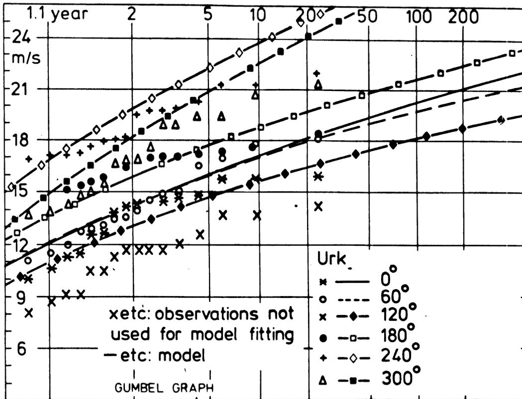
Fig. 20.17 Annual azimuth-sector maximum hourly wind speed for Urk as observed and as computed from the model independent of these observations.
