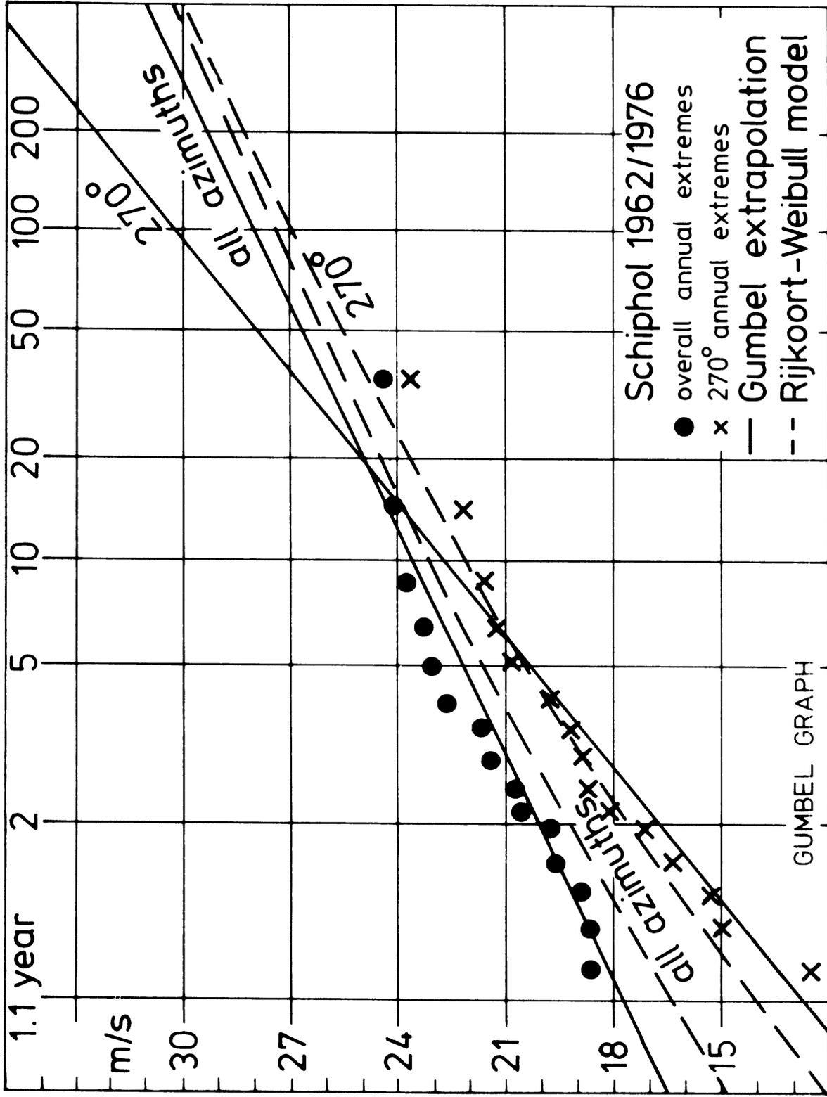
Fig. 23 Annual extreme values of hourly average wind observed at Schiphol, both for all azimuth and only for azimuth sector 255°-285°, with fitted Gumbel-Lieblein lines and computed model curves.
