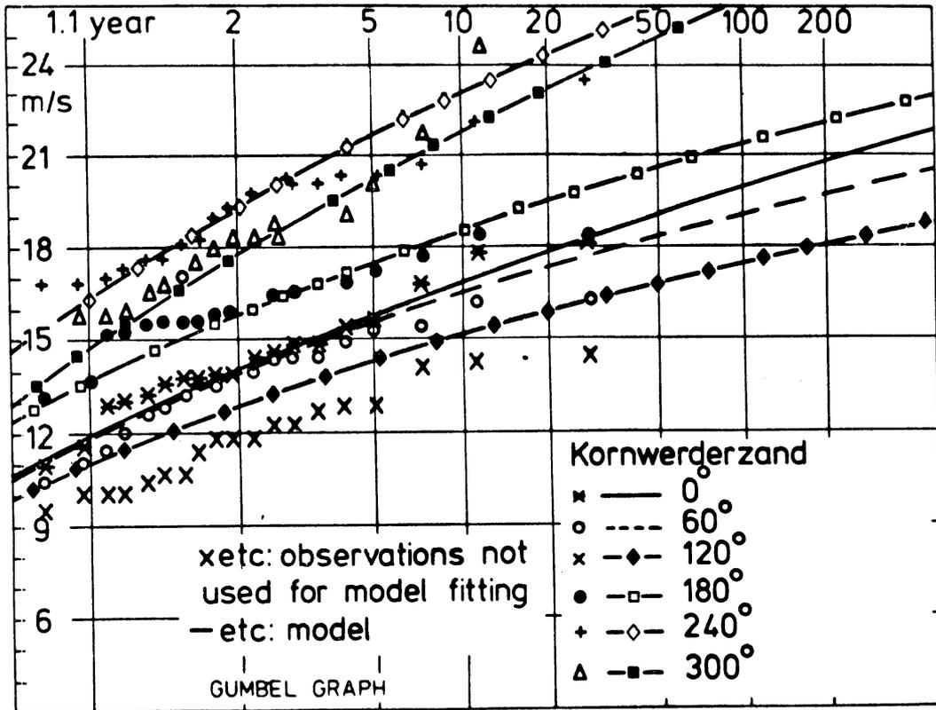
Fig. 20.15 Annual azimuth-sector maximum hourly wind speed for Kornwerderzand as observed and as computed from the model independent of these observations.
