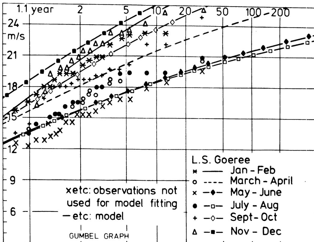
Fig. 20.10 Seasonal maximum hourly wind speed in successive years for Lightvessel Goeree as observed and as computed from the model independent of these observations.
