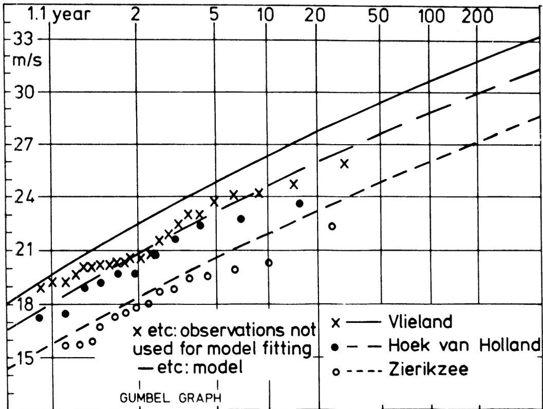
Fig. 20.3 Annual maximum hourly wind speed for Vlieland, Hoek van Holland and Zierikzee as observed and as computed from the model independent of these observations.
