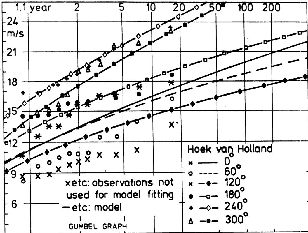
Fig. 20.13 Annual azimuth-sector maximum hourly wind speed for Hoek van Holland as observed and as computed from the model independent of these observations.
