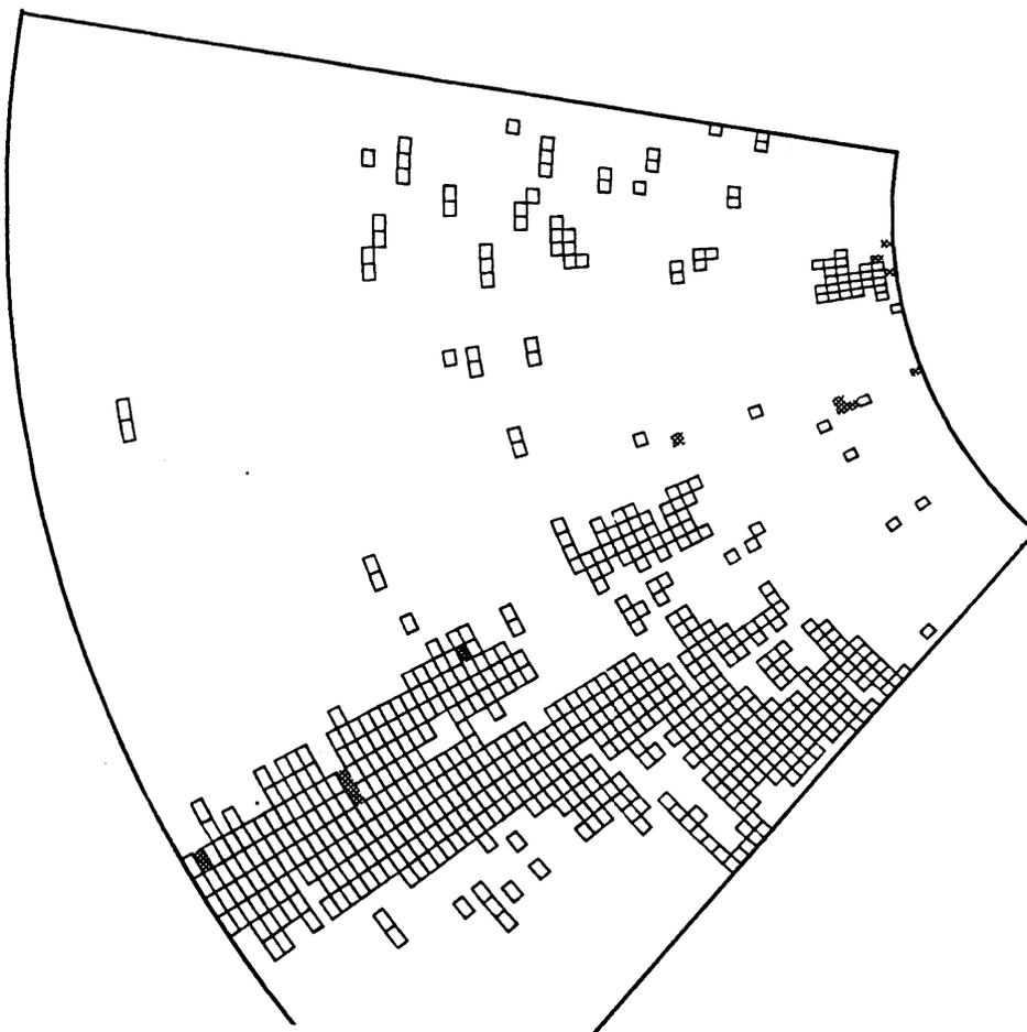
Fig.4. Radar picture sector for range 68-220 km in a clutter situation (Jan.11, 1992). The empty boxes show pixels that will be removed.
