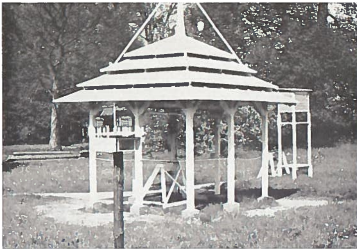
FIG. 2. Big screen for climatological measurements: behind it a normal STEVENSON-screen, on the foreground a small screen (mentioned in Ch. II) placed on a pole
