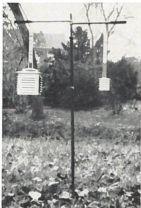
FIG. 1. The small plastic (vinydur) screen (for one thermometer) and the original smaller metal type with single louvres
