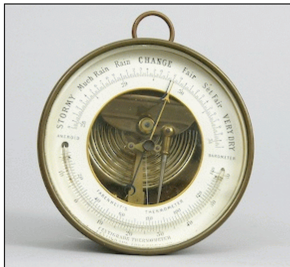
Figure 5: Aneroid barometer as used on clipper ships around 1850
