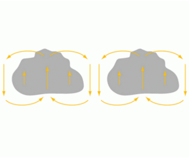
Figure 3-11 Scheme of vertical circulation and cloudiness in Closed Cell Convection
