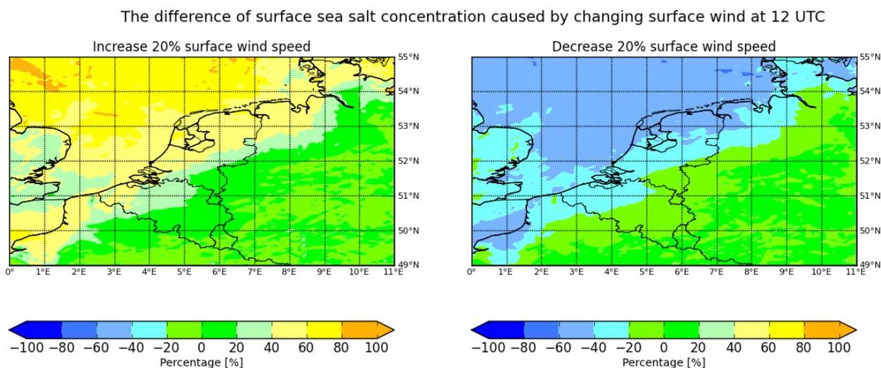
Figure 24. The difference in surface sea salt concentration between the sensitivity experiments and the control result at 12 UTC for the period 25 to 31 July (Unit: %). (a) Increasing surface wind speed by 20%. (b) Decreasing surface wind speed by 20%.
