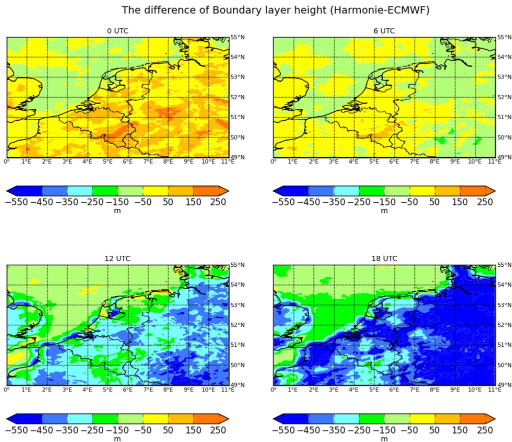
Figure 14 The difference of average boundary layer height (m) between ECMWF and Harmonie over the whole domain at 4 times (0, 6, 12, 18 UTC).
