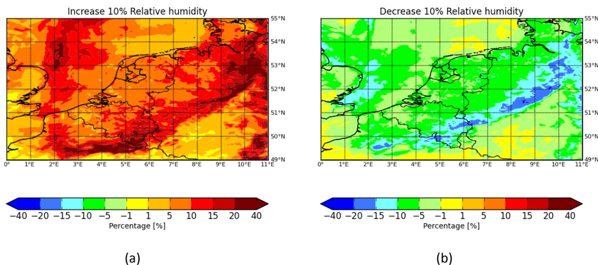
Figure 20. The difference in surface  $\text{PM}_{10}$  concentration between the sensitivity experiments and the control result at 12 UTC for the period 25 to 31 July (Unit: %). (a) Increasing relative humidity by 10%. (b) Decreasing relative humidity by 10%.
