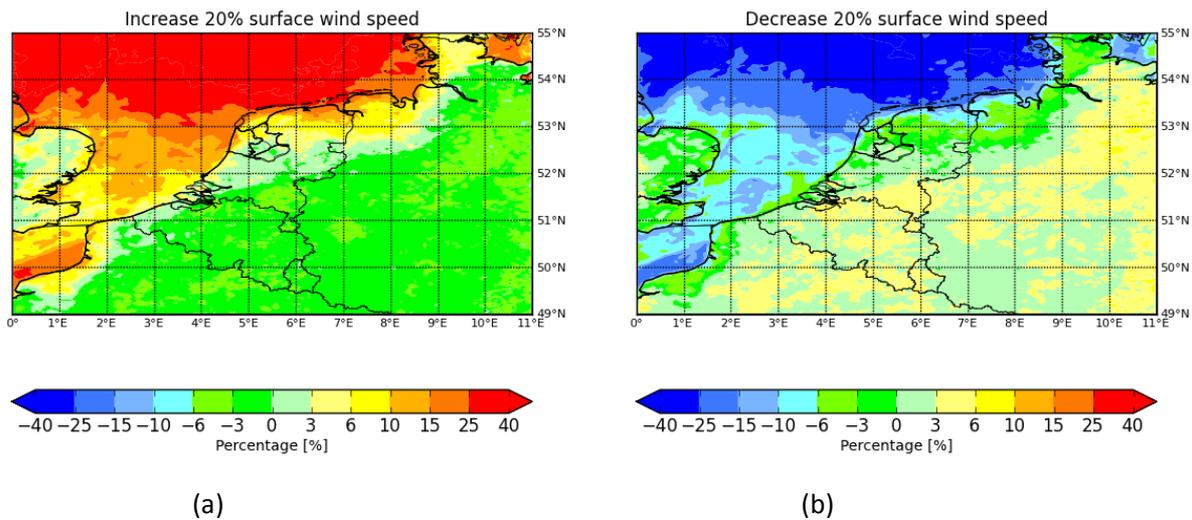
Figure 22. The difference in surface PM10 concentration between the sensitivity experiments and the control result at 12 UTC for the period 25 to 31 July (Unit: %). (a) Increasing surface wind speed by 20%. (b) Decreasing surface wind speed by 20%.
