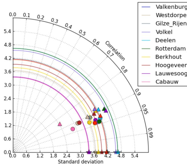
**Figure 5. Taylor diagram of surface temperature [K] during period June to August, 2012. The stars are the observations; the circles correspond to ECMWF, and the triangles to Harmonie. The standard deviation is the radial distance to the origin. The distance between observation and model represents the pattern RMSD (in the same units as standard deviation which is K). The correlation coefficient between model and observation is given by the azimuthal position.**
