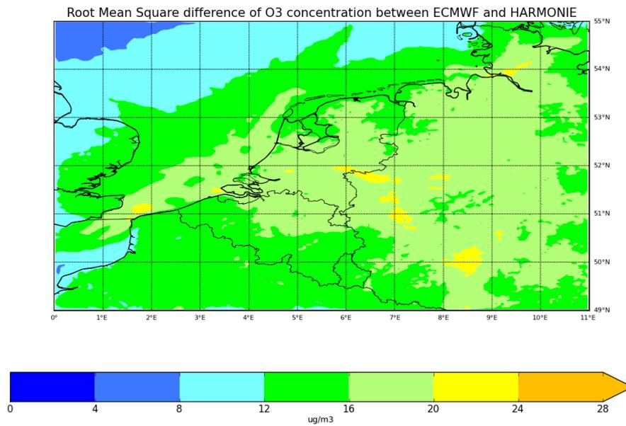
Figure 18. O<sub>3</sub> RMS difference between the two LOTOS-EUROS simulations driven by ECMWF and Harmonie.
