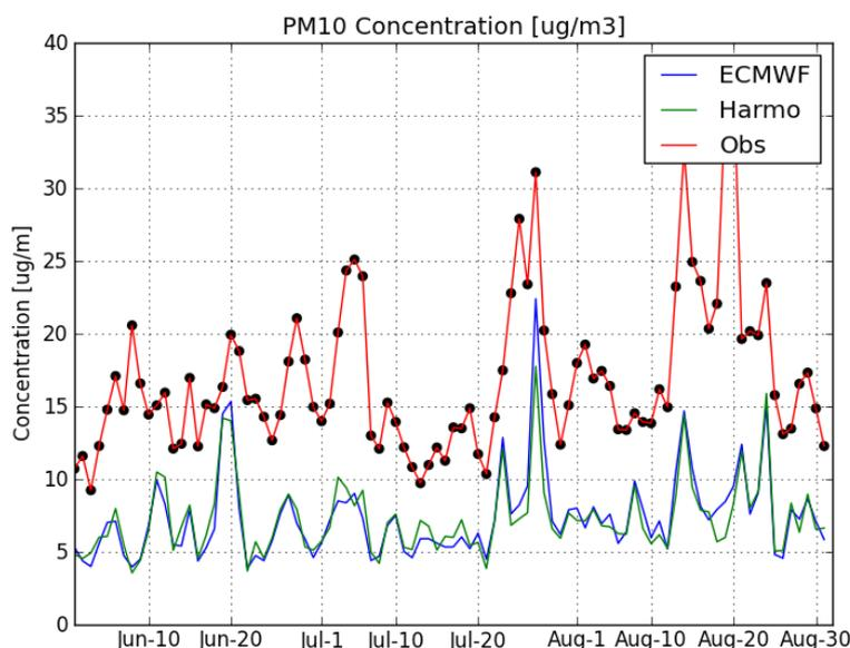
Figure 15. The time series of PM10 concentration from June to August 2012 at 8 selected stations. The red line is observation data. The blue and green lines present the simulations driven by ECMWF and Harmonie respectively.
