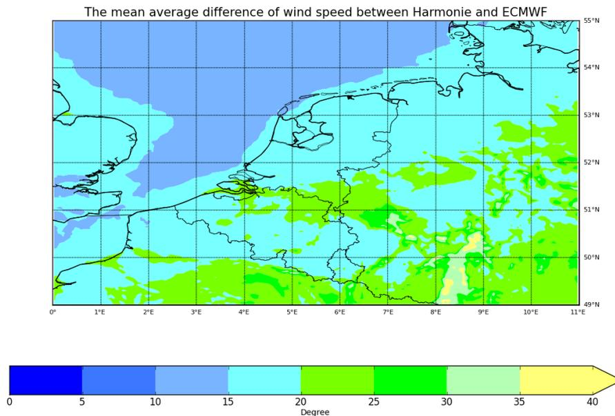
Figure 12. The mean absolute difference in wind direction between the ECMWF and Harmonie from June to August, 2012.
