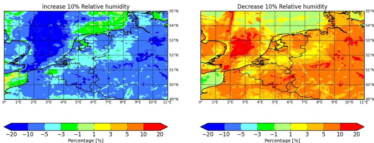
Figure 21. The difference in surface  $\text{NH}_3$  concentration between the sensitivity experiments and the control result at 12 UTC for the period 25 to 31 July (Unit: %). (a) Increasing relative humidity by 10%. (b) Decreasing relative humidity by 10%.
