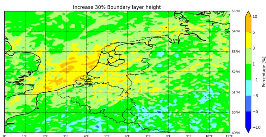
Figure 26. The difference in surface  $O_3$  concentration between the sensitivity experiments and the control result at 12 UTC for the period 25 to 31 July (Unit: %). The sensitivity run is increasing the boundary layer height by 30%.
