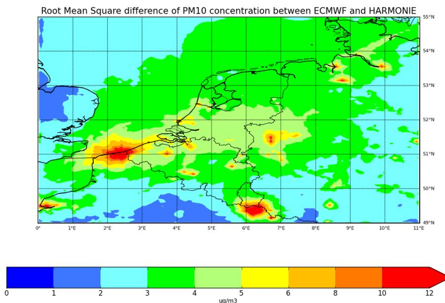
Figure 16. PM10 RMS difference between the two LOTOS-EUROS simulations driven by ECMWF and Harmonie.
