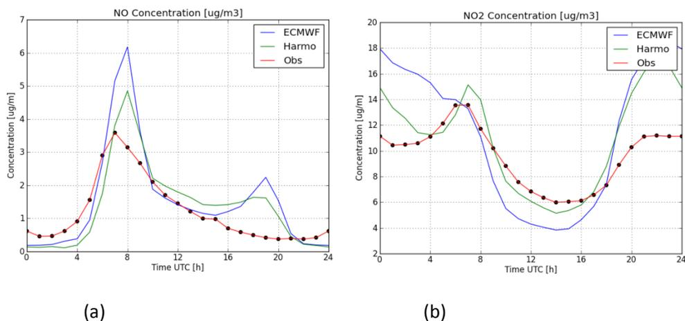
**Figure 19.** The average daily evolution of NO (a) and NO<sub>2</sub> (b) concentration at the 8 Dutch stations for the period June to August, 2012. The red line is observation data. The blue and green lines present the simulations driven by ECMWF and Harmonie respectively.
