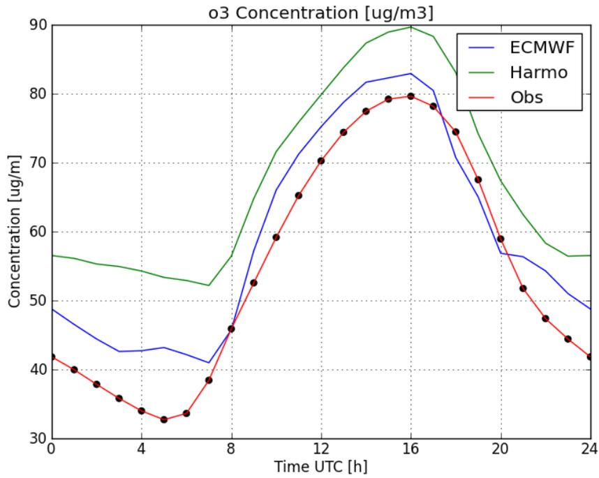
Figure 17. The average daily evolution of ozone at the 8 Dutch stations from June to August, 2012. The red line is observation data. The blue and green lines present the simulations driven by ECMWF and Harmonie respectively.
