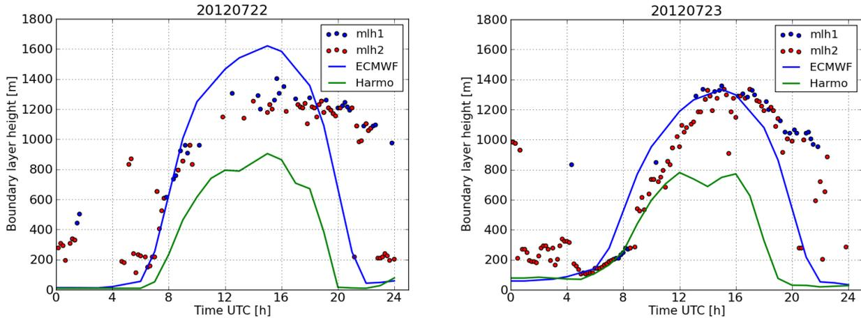
Figure 13 The diurnal boundary layer height. (a) 22 July, 2012; (b) 23 July, 2012. ( There are two ceilometers to detect the boundary layer height shown by dots. There are four levels of observation data quality. Only the observation data with highest quality level are used.)
