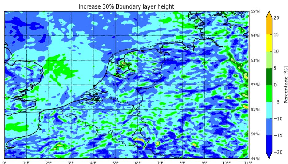
Figure 25. The difference in surface PM10 concentration between the sensitivity experiments and the control result at 12 UTC for the period 25 to 31 July (Unit: %). The sensitivity run is increasing the boundary layer height by 30%.
