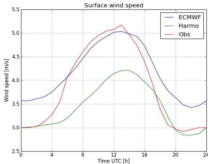
Figure 10. The average diurnal evolution of surface wind speed during the period from June to August 2012. The red line is observation data. The blue and green lines present the ECMWF and Harmonie respectively.
