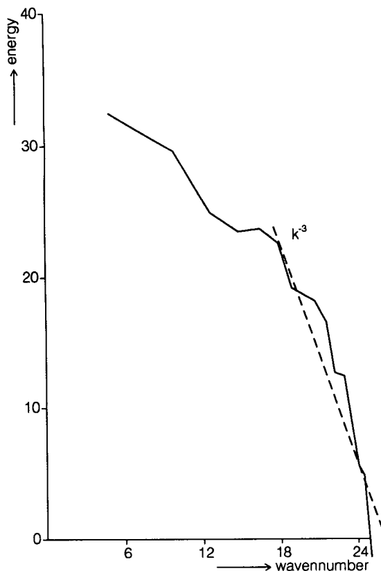
FIG. 1. Kinetic energy spectrum at day 30 in 10^{-3} \text{ m}^3 \text{ s}^{-2} .
