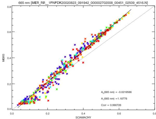
Fig. 3. Correlation at 665 nm between SCIAMACHY and MERIS reflectances for the pixels shown in Fig. 2. The color shows the SCIAMACHY scanning angle between 0 and 30 degrees (coded red-green-blue).
