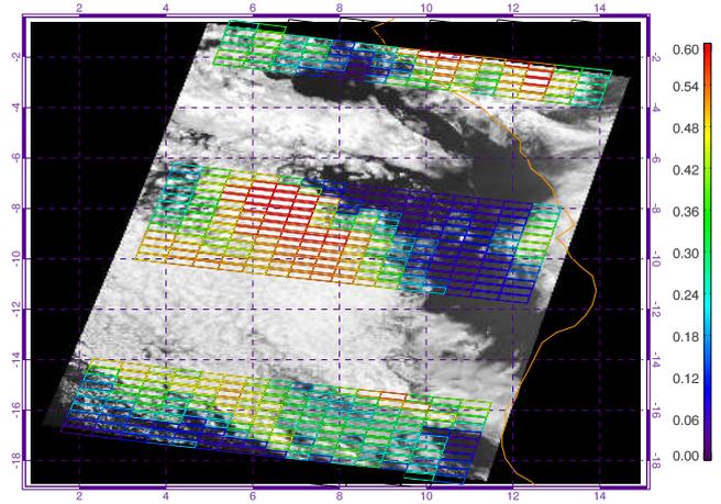
Fig. 2. Common projection for a MERIS image (gray, background) and SCIAMACHY data (color, foreground). The color bar (right) shows the SCIAMACHY reflectance at 665 nm.
