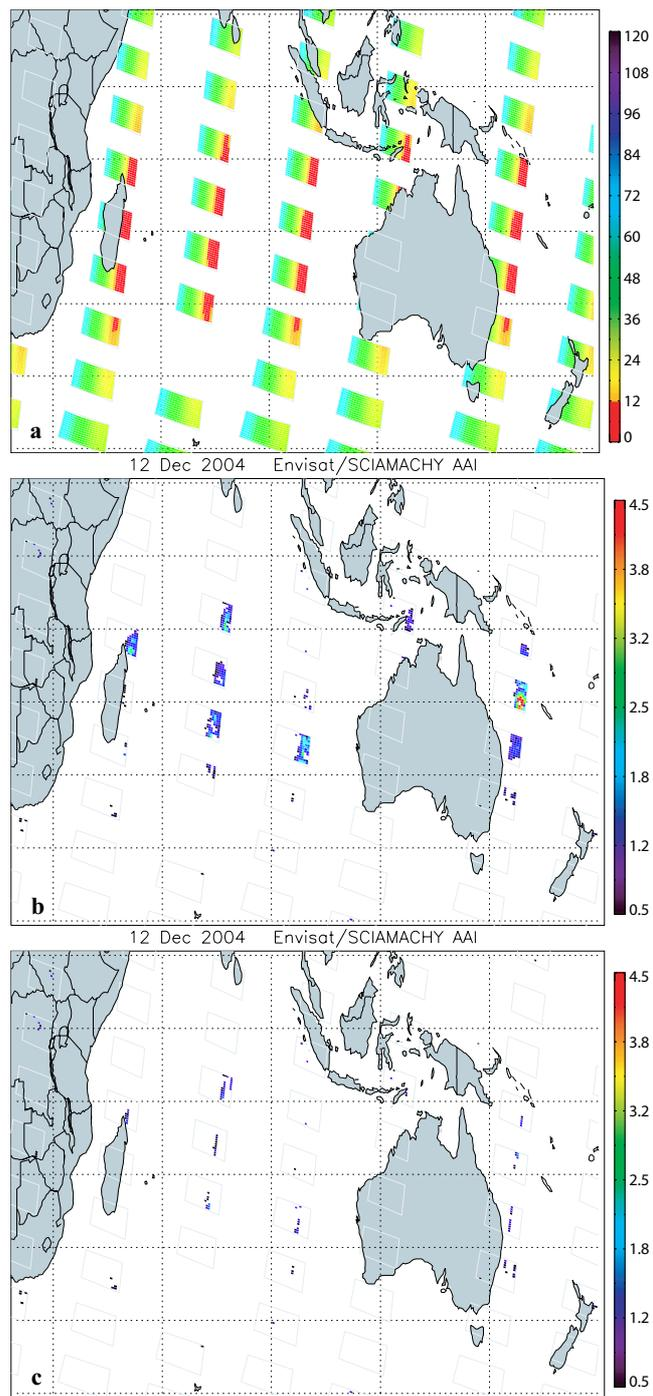
**Fig. 4.** SCIAMACHY SC-AAI on 12 December 2004 over the Indian Ocean, Indonesia and Australia, and the south-western Pacific. a) Sun glint deviation angle of SCIAMACHY ocean pixels. The sun glint deviation angle has a smooth scale, but all pixels satisfying the sun glint condition, i.e. having a sun glint deviation angle lower than  $12^\circ$ , are marked in red. b) SC-AAI without sun glint mask. c) SC-AAI with all ocean pixels with a sun glint deviation angle lower than  $12^\circ$  removed.
