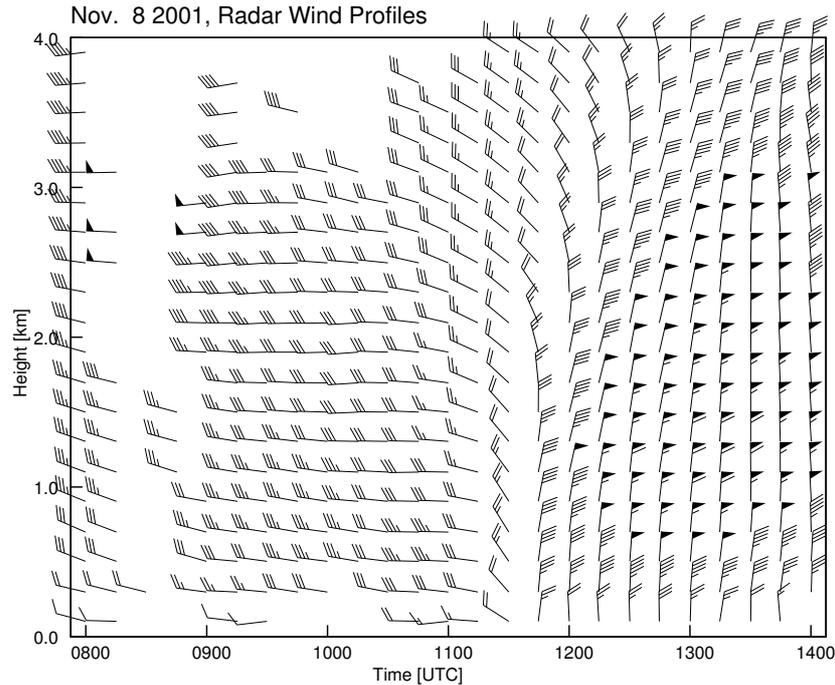
Figure 3: A time series of wind profiles from the De Bilt radar of the Netherlands Royal Meteorological Institute (KNMI). Wind speed and direction are indicated by wind vanes. Each full barb represents a wind speed of 5 m/s and each triangle a wind speed of 25 m/s.
