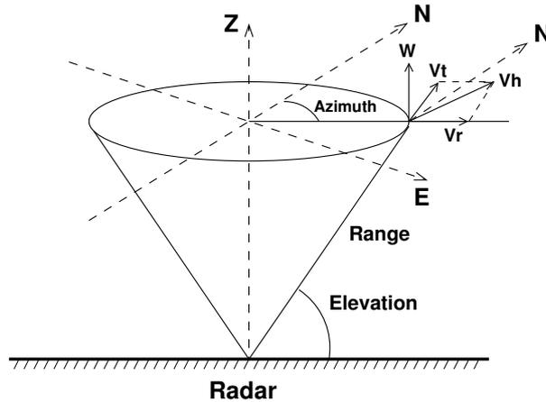
Figure 2: Radar geometry for measuring wind profiles.
