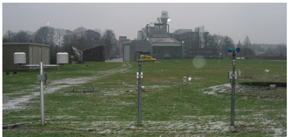
Figure 6: Instruments at the operational site DB260. To the left the KNMI multi-plate radiation shield for measuring temperature and to the right the cup anemometer. Both instruments operate at 1.5 m above ground level. The 4 parallel locations are equipped with the same instruments.
