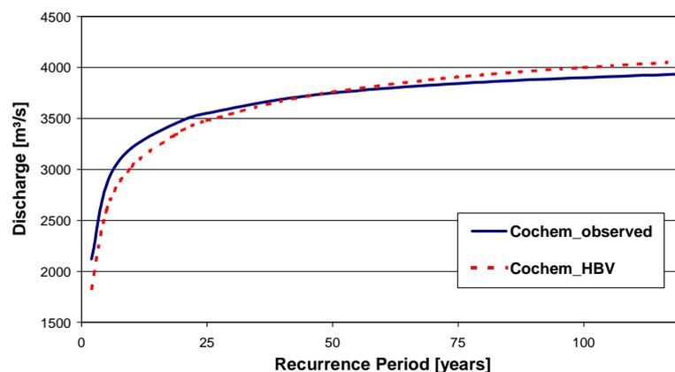
Figure 3-3: Log Pearson Type III distribution estimated with the maximum-likelihood method on the basis of measured and simulated annual peak discharges at gauge Cochem/Moselle 1962-1997
