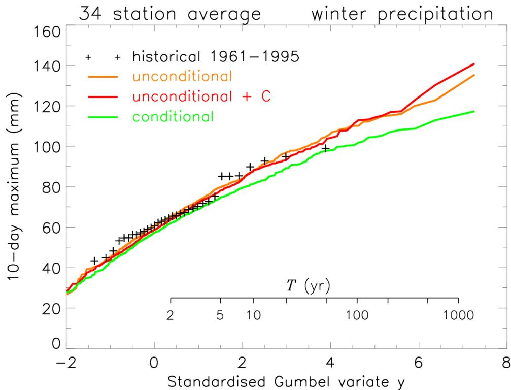
Figure 3: Gumbel plots of 10-day winter precipitation maxima for observed and simulated data (runs of 1000 years)
