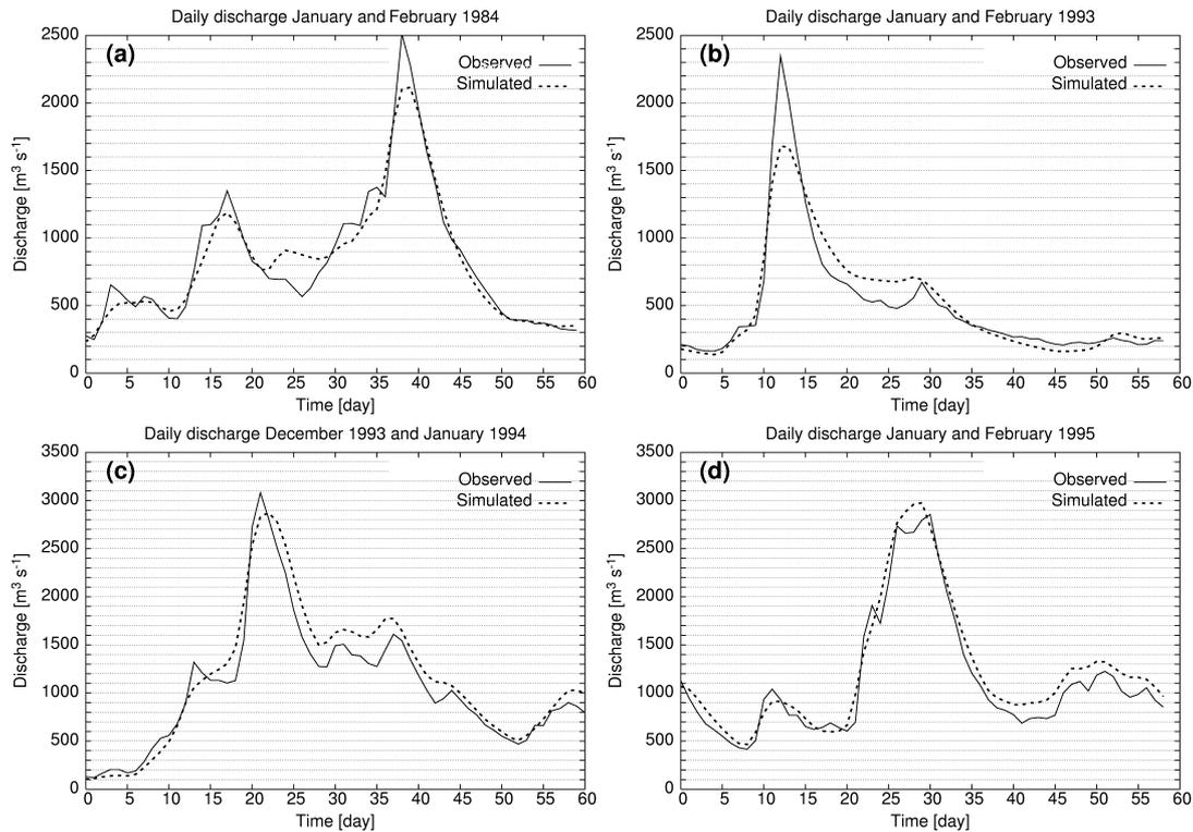
**Fig. 6** Observed (solid) and simulated (dashed) daily discharge at Borgharen around the winter maxima of (a) 1984, (b) 1993, (c) 1994 and (d) 1995.
