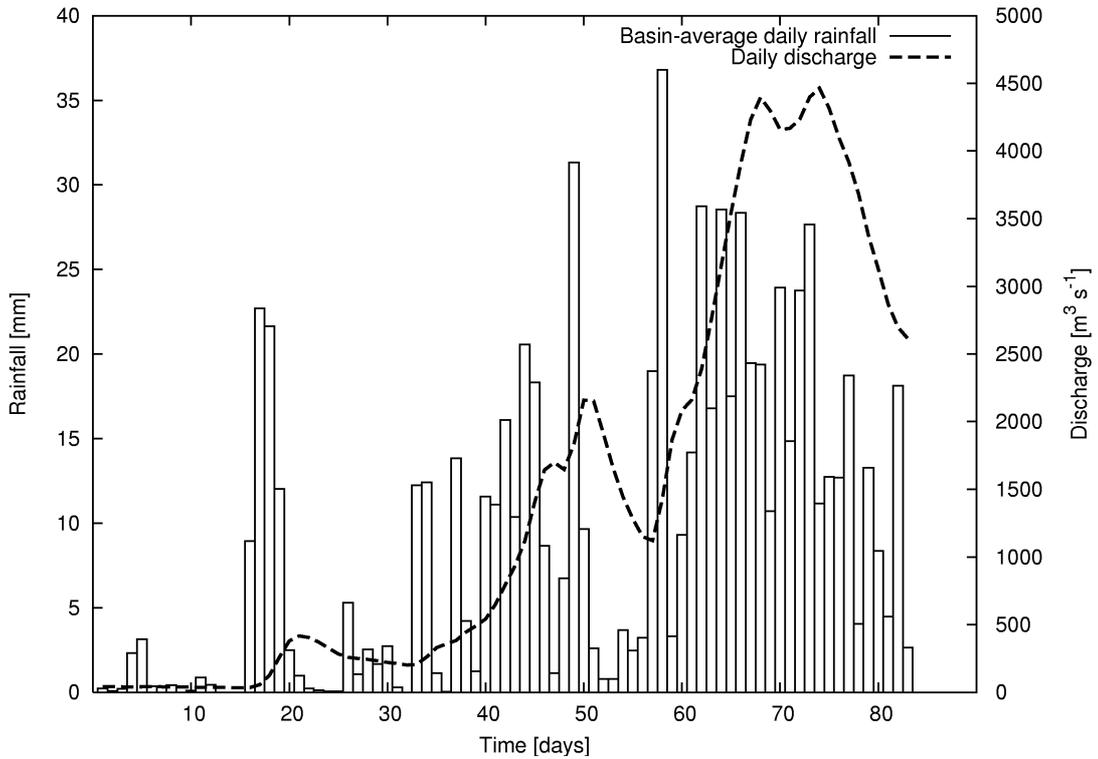
**Fig. 7** The daily discharge (dashed curve) around the highest discharge maximum ( $4464 \text{ m}^3 \text{ s}^{-1}$ ) in the HBV simulation driven by Sim61 and the corresponding daily rainfall (bars).
