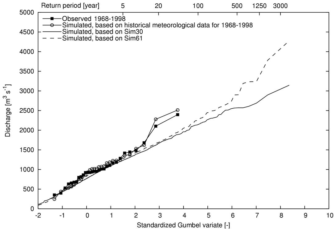
**Fig. 9** Winter maxima of the observed 10-day average discharge at Borgharen and those simulated using respectively historical meteorological data or data from Sim30 and Sim61.
