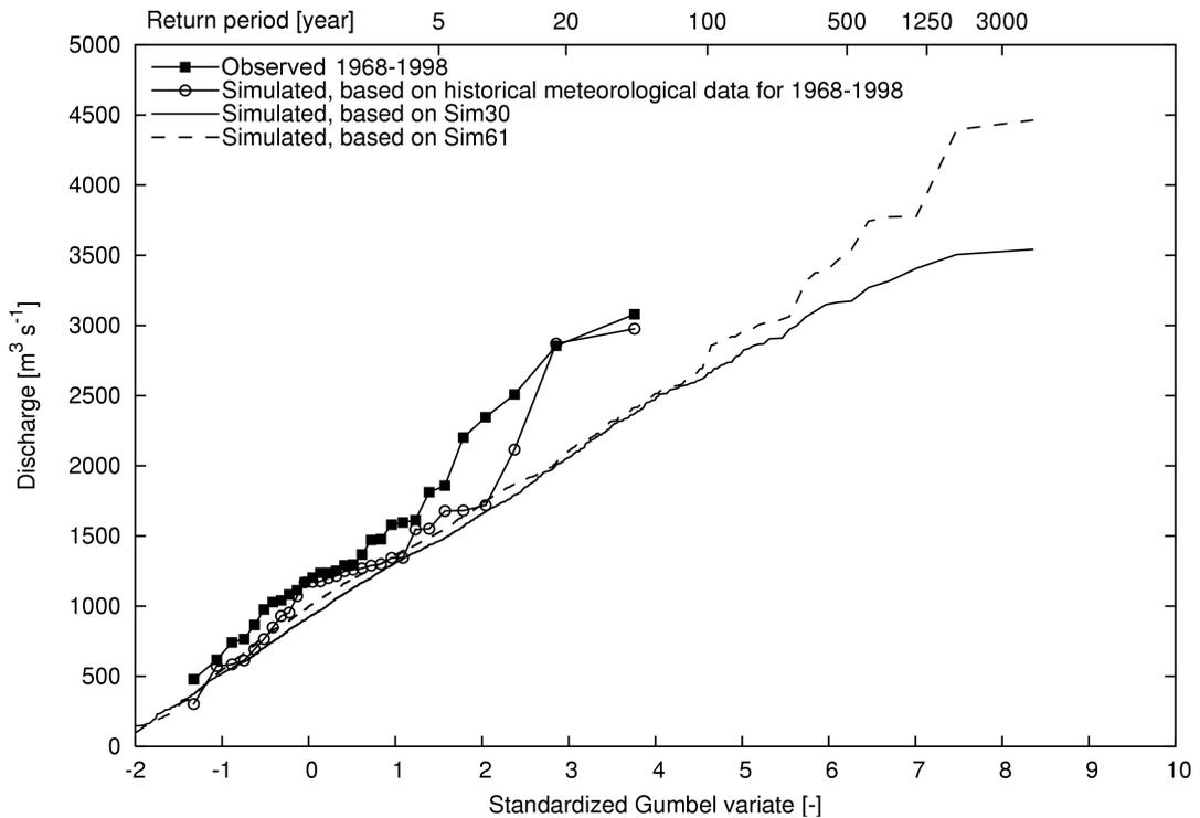
**Fig. 8** Winter maxima of the observed daily discharge at Borgharen (1968–1998) and the simulated daily discharge based on the historical meteorological data for 1968–1998, Sim30 and Sim61.
