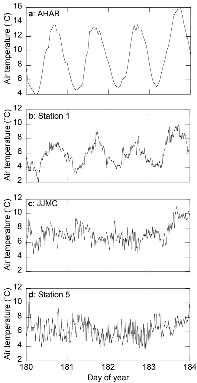
Figure 4: Air temperature for four clear-sky days at AHAB (a), Station 1 (b), JJMC (c) and Station 5 (d) shown in Figure 1. Measurements at AHAB are hourly averages, and at the other stations 15-minute averages.
