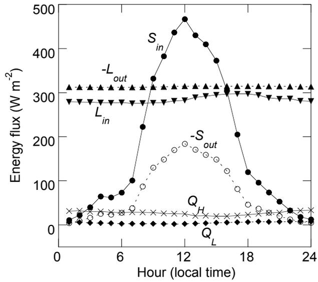
Figure 7: Mean daily cycle in incoming ( $S_{in}$ ) and reflected ( $S_{out}$ ) solar radiation, incoming ( $L_{in}$ ) and outgoing ( $L_{out}$ ) longwave radiation and the sensible ( $Q_H$ ) and latent ( $Q_L$ ) heat fluxes. The daily fluctuations are averages over the period 27 May to 20 August 2004.
