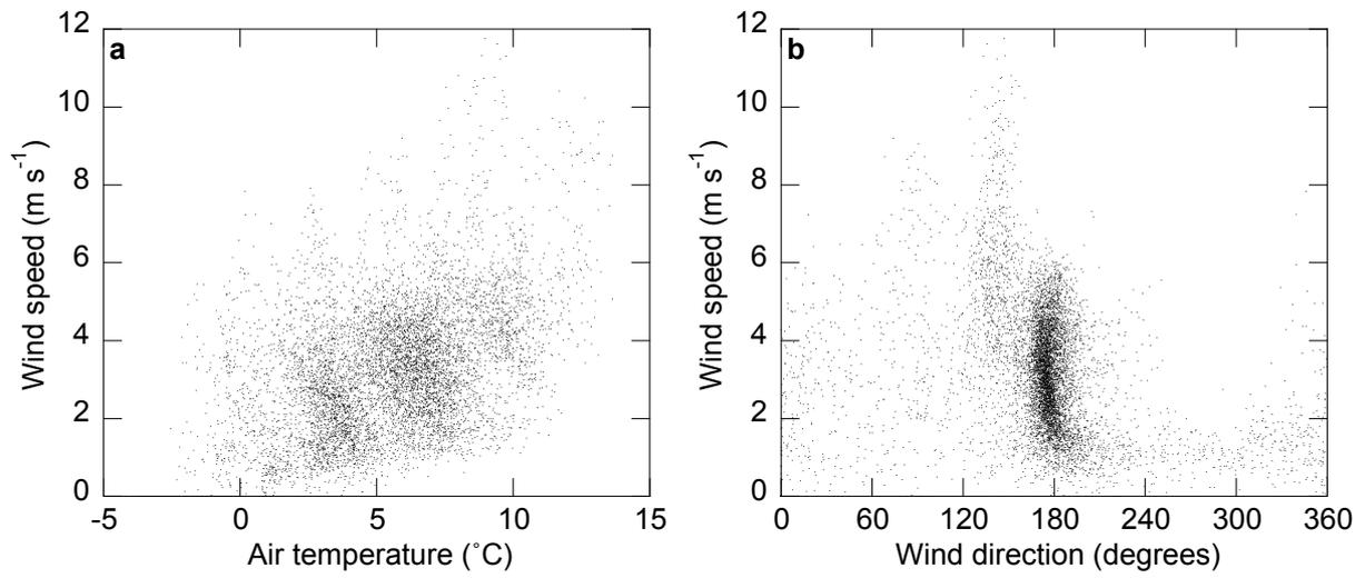
Figure 5: Wind speed at JJMC as function of air temperature (a), and wind direction (b) for the period 27 May to 20 August 2004 (15-minutes averages).
