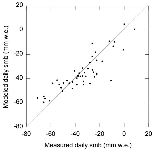
*Figure 9: Modeled (derived from the surface energy balance) versus measured (derived from sonic height ranger and ablation stake data) daily specific mass balance (smb).*
