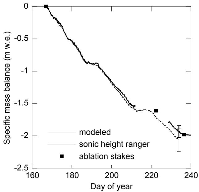
Figure 8: Specific mass balance as measured by the sonic height ranger and the ablation stakes (squares), and modeled from the surface energy balance. All records start at 15 June (JD 165) and the modeled specific mass balance ends at 20 August 2004 (JD 233). The error bars at 20 August indicates the accuracy of the modeled (thin error bar; section 6.2) and measured (thick error bar; section 5.3) specific mass balance.
