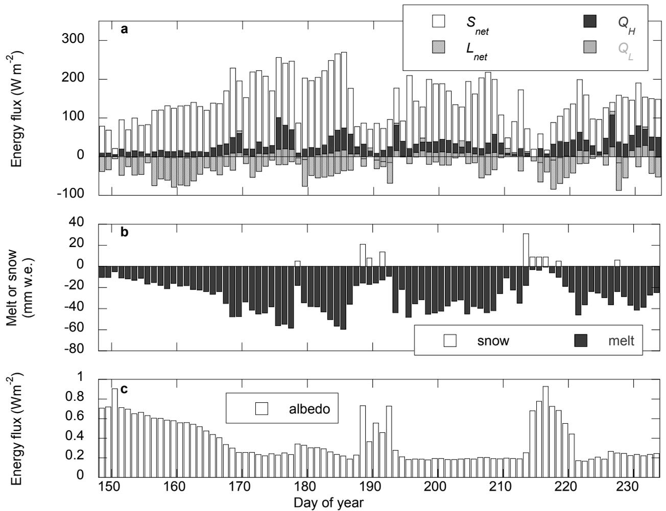
Figure 6: (a) Daily means of the net solar radiation ( $S_{net}$ ), net longwave radiation ( $L_{net}$ ) and the sensible ( $Q_H$ ) and latent ( $Q_L$ ) heat fluxes, (b) daily surface melt and snowfall and (c) daily mean albedo for the period 27 May to 20 August 2004 (JD 148-233).
