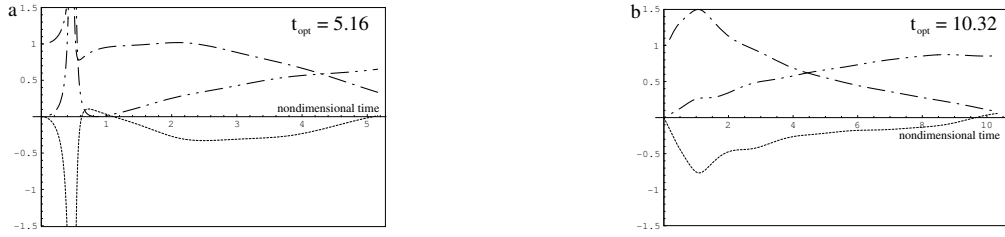
Fig. 11: The time-evolution of the different surface projection coefficients for (a) the t_{opt} = 5.16 and (b) t_{opt} = 10.32 (right) SV with M = 40 PV anomalies. Initial norm total kinetic energy. Norm: total kinetic energy. (\langle \psi_{pv}, \psi_{pv} \rangle_L / \|\psi_{sv}\|^{-2})|_{z=0} (dash-dot), (2\langle \psi_{pv}, \psi_{\theta} \rangle_L / \|\psi_{sv}\|^{-2})|_{z=0} (full) and (\langle \psi_{\theta}, \psi_{\theta} \rangle_L / \|\psi_{sv}\|^{-2})|_{z=0} (dash-dot-dot).
