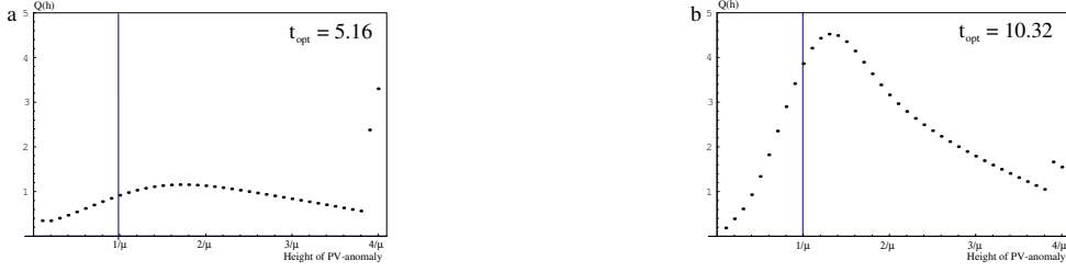
Fig. 12: Amplitudes of the PV-maxima for (a) the t_{opt} = 5.16 SV and (b) t_{opt} = 10.32 SV. The anomalous large amplitude of the PV at the two topmost levels is the effect of truncating the vertical domain at z = 4/\mu , and in some sense summarized the mean effect of all modes above that level.
